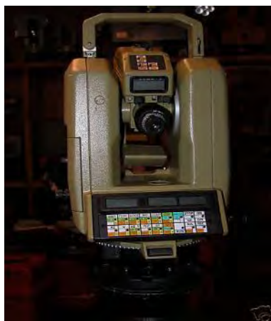
Figura 10. Primele teodolite electronice performante a. WILD T2002, b. Kern E2, c. Leica T3000 (197)
