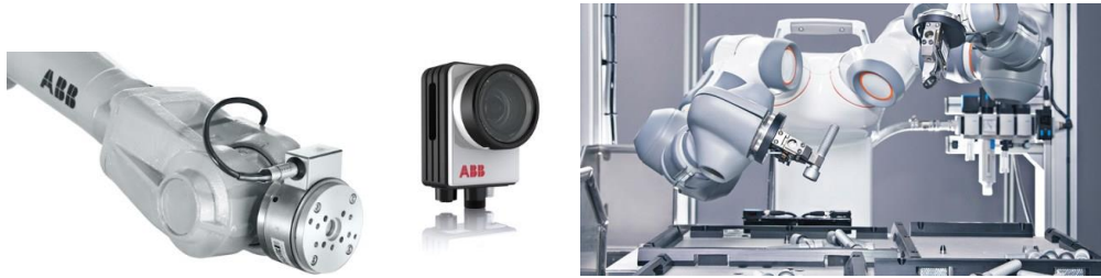
Fig. 1.1.8. Example of force and vision systems embedded in the robot arms (courtesy ABB)
