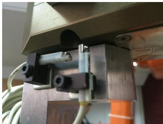
Fig. 4.2.4. Magnetic sensor and magnets mounted on gripper
