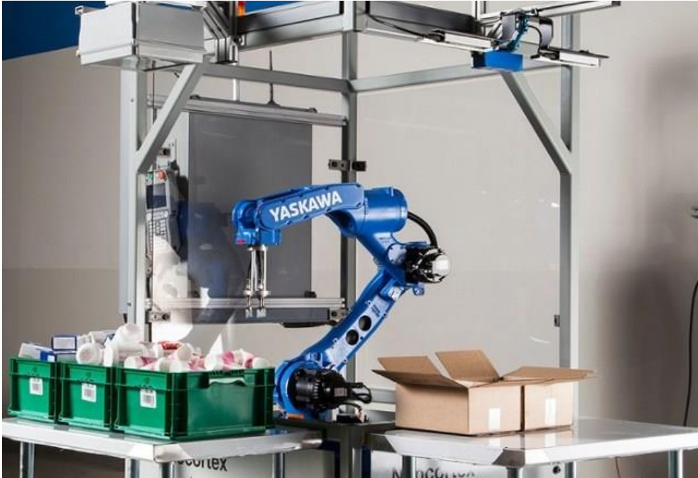
Figure 1.1.11. Plug-and-play intelligent adaptive robotic cell (courtesy Yaskawa Motoman and Universal Logic)
