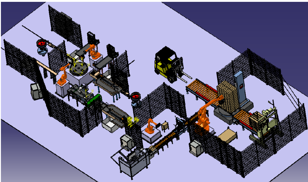
Fig. 3.3.2. 3D virtual prototype of a robotic production system layout (Catia screenshot)
