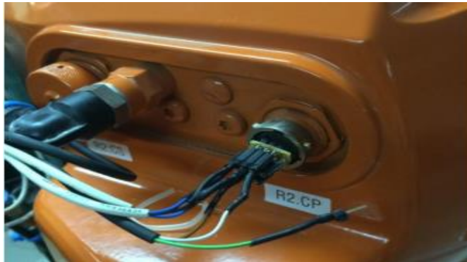
Fig. 4.2.19. Third robot joint with R2-CP and R2-CS jack connectors
