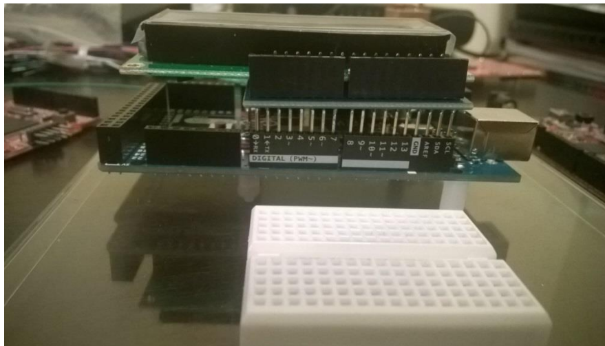
Fig.III.5. Connecting the LCD shield to Arduino
