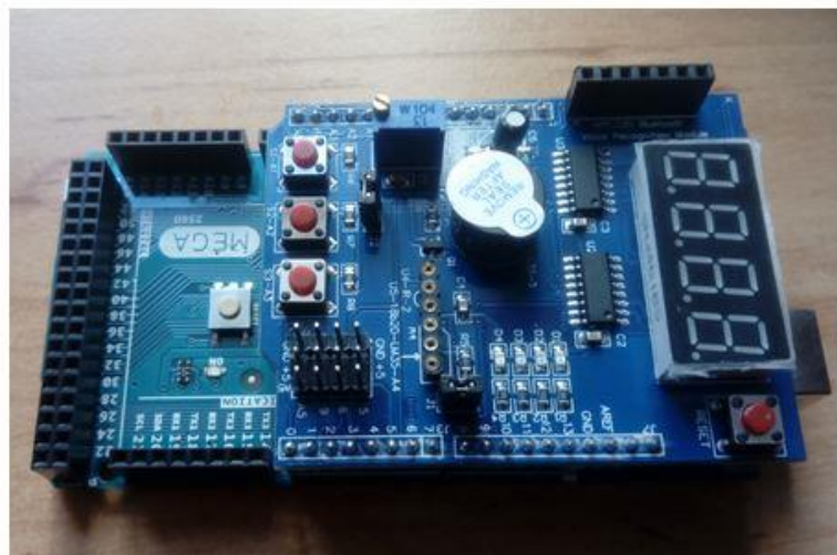
Fig.II.9, Fig.II.10 – The learning Shield and Arduino
