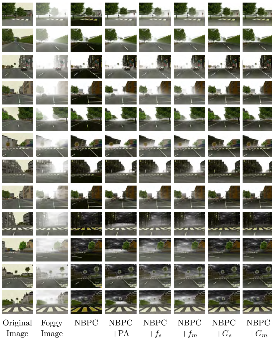
Figure 4.21: Contrast restoration results on synthetic images. From left to right, the original image without fog, the original image with synthetically added fog and the restoration results with the following algorithms: NBPC, NBPC+PA [85], NBPC + f_s , NBPC + f_m , NBPC + G_s and NBPC + G_m . The used parameters are k = 15 , p = 0.99\% and a = 3.5
