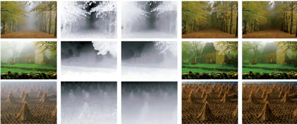
Figure 4.5: The results of haze removal using the method of He et al. [79]. From left to right we present the input hazy image, estimated transmission map before soft matting, estimated transmission map after soft matting, restoration result without soft matting and restoration result with soft matting.
