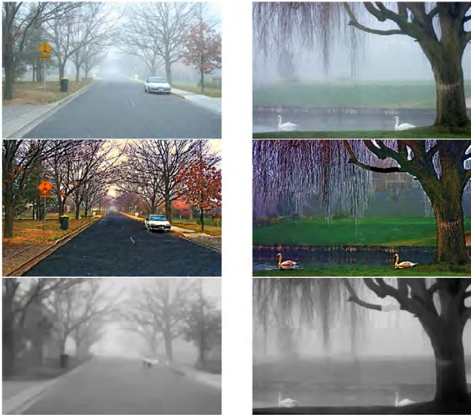
Figure 4.3: Top: input image, middle: the result obtained by Tan's method [75], bottom: the air light. Images taken from [75]
