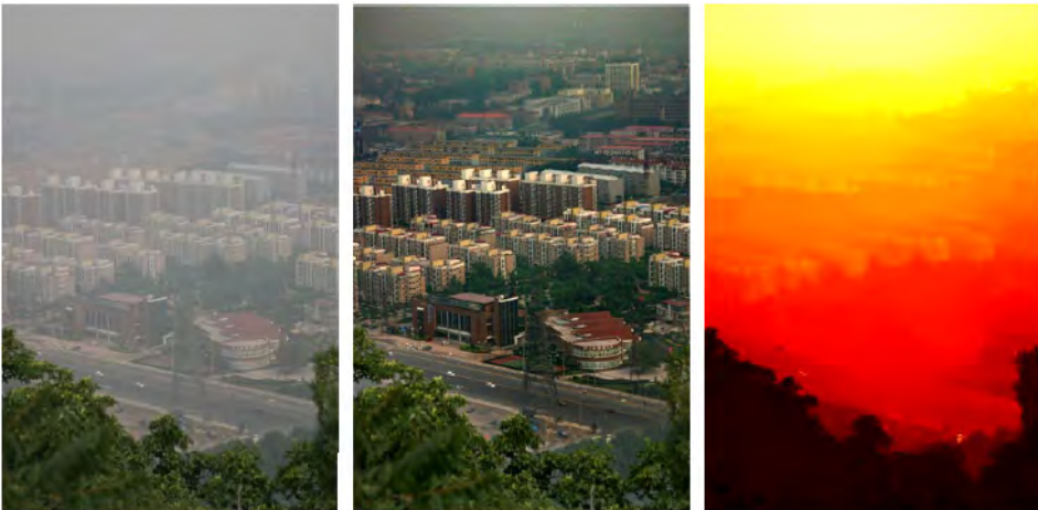
Figure 4.4: The results of haze removal using the method of He et. al. [79]. From left to right we present the input hazy image, the restoration result and the approximation of the recovered depth map.
