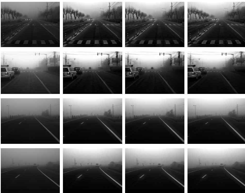
Figure 4.15: Image Enhancement Results on Traffic Images. From Left to right, the original image captured in fog conditions, and the three images enhanced with the proposed method by using the squared median filter, the median filter along lines and the median filter along columns.
