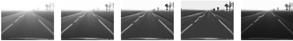
Figure 4.9: The results of contrast restoration with the method described in [80] on traffic scenes with different parameters. From left to right the original foggy image and the results with: p = 0.7 and sv = 61 , p = 0.9 and sv = 61 , p = 0.98 and sv = 61 , p = 0.90 and sv = 21
