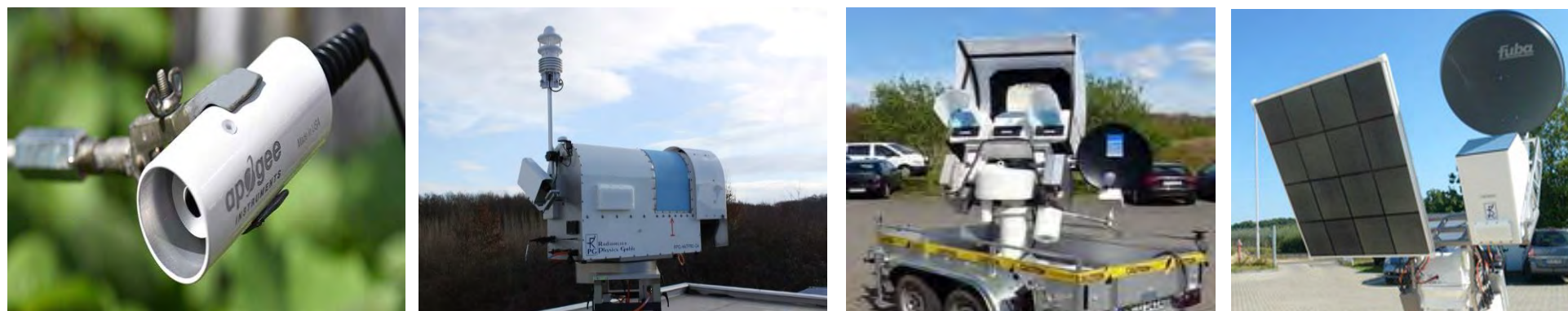
Figura 3.13. Exemple de Radiometre utilizate ca senzori pasivi: a. Infrared Radiometers produs de Apogee Instruments, Inc.[70], b. Unpolarized Radiometers Humidity And Temperature PROFilers produs de RPG Radiometer Physics GmbH[71], c. Dual Polarisation Radiometers- Dual Polarisation Rain Radiometer (DP-RR) for thick cloud and rain LWP[71], d. Dual Polarisation Surface Radiometers[71]
