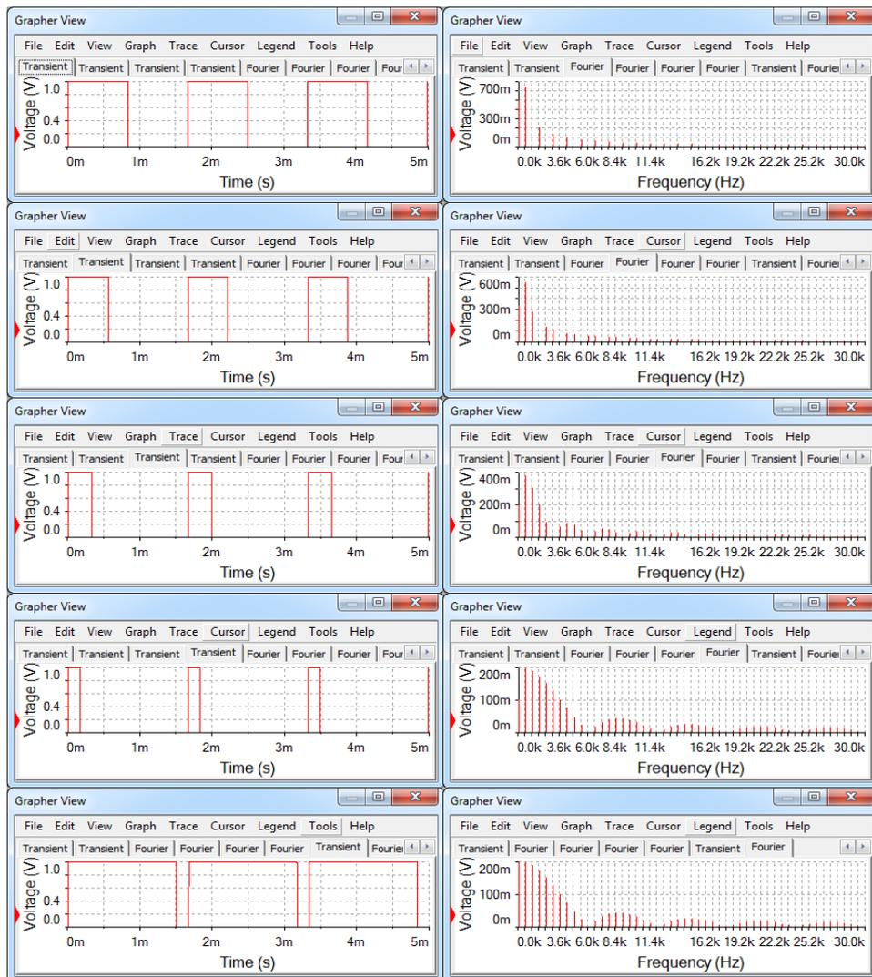
**Figure 1.2** Left: 600Hz rectangular signals with various duty factors (from top to down: 1/2, 1/3, 1/5, 1/10, 9/10).
