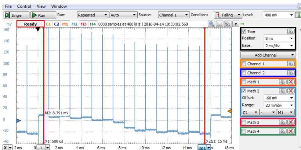
**Figure 3.12** The weighted resistor network output voltage error
