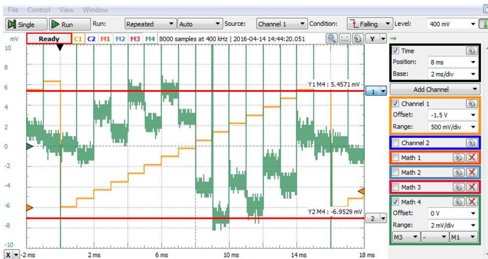
**Figure 3.15** Measuring the absolute integral linearity error
