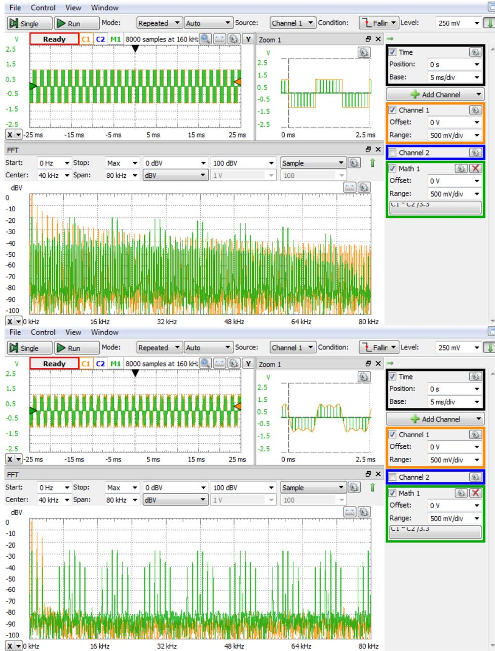
**Figure 1.13** Ideal sampling on rectangular (up) and filtered (down) signal
