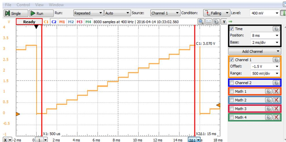
**Figure 3.10** The weighted resistor network output voltage ramp
