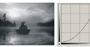
$\gamma > 1$ : gamma decoding/expansion
