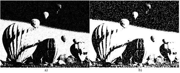
Fig. 7.5 Example of the erosion (object = black / background = white): a) Original image A; b) The result image:  $\mathbf{A} \Theta \mathbf{B}$
