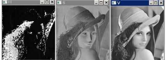
b) Results on *Lena\_24bits.bmp* (24 bits/pixel) **Fig. 2.6** Examples of RGB to HSV conversion
