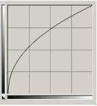
$\gamma < 1$ : gamma encoding/compression
