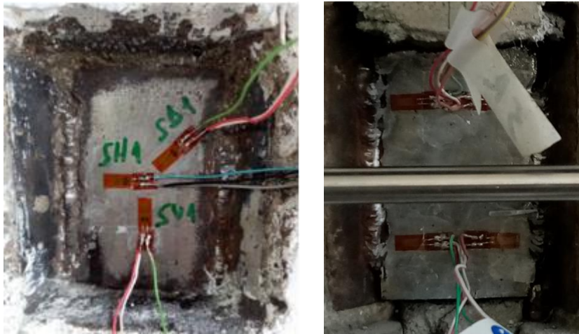
Figure 2-5 Strain gauges on the welded plates (left image: SA1; right image: SA2)
