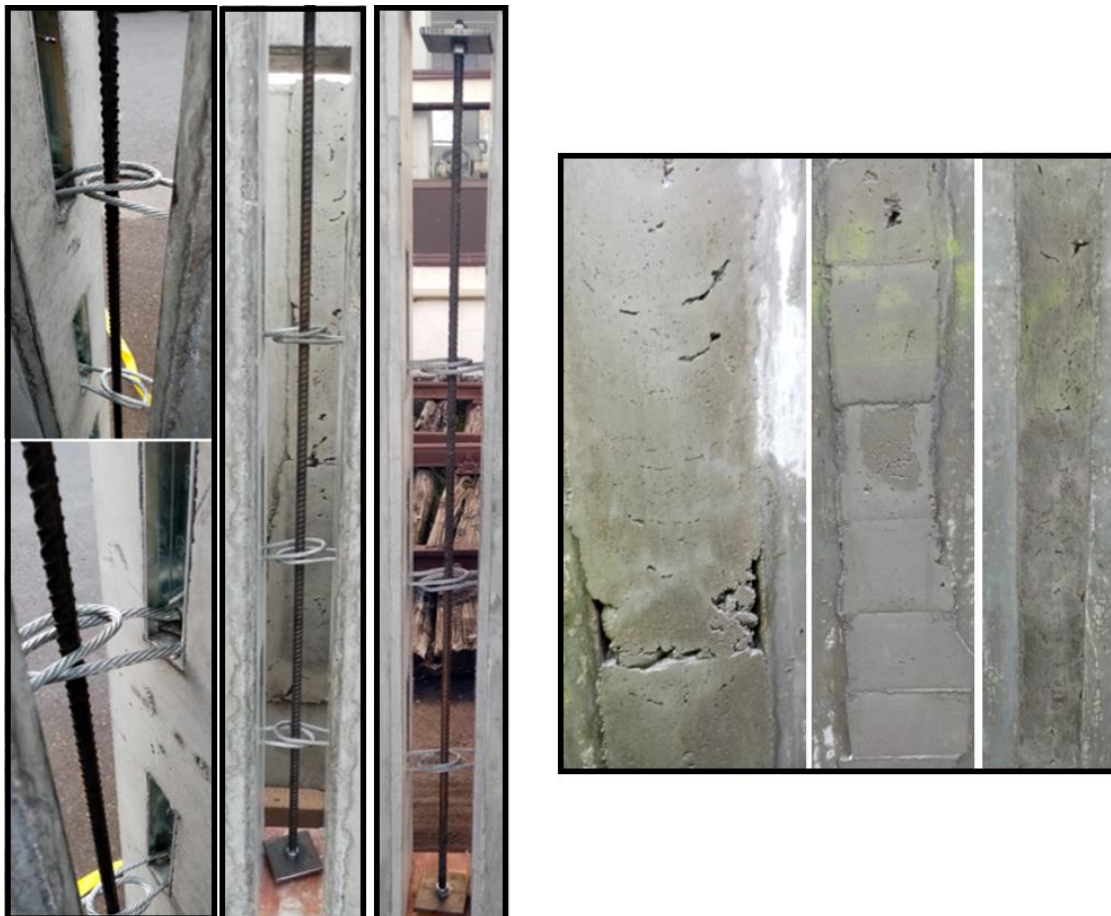
Figure 4-4 Test specimens before (left images) and after (right images) joint casting
