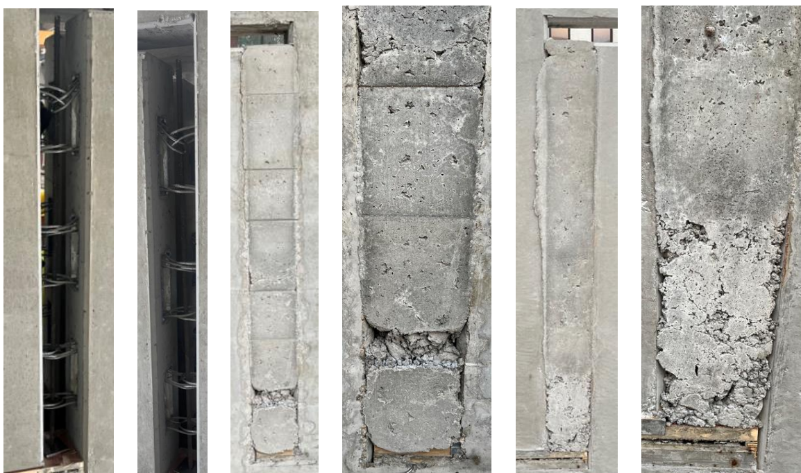
Figure 4-33 Test specimens before (left images) and after (right images) joint castings
