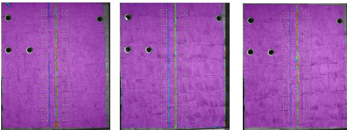
Figure 4-43 Observed failure mechanisms after failure (from left to right). Peak loads for Test 1: 178.8 kN; Test 2: 124.7 kN; Test 3: 102.2 kN
