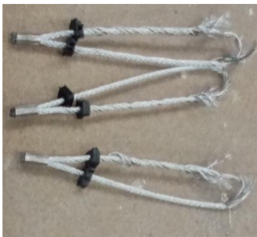
Figure 4-41 Wire loops after testing (preloaded by \approx 0.5kN to straighten the wires)
