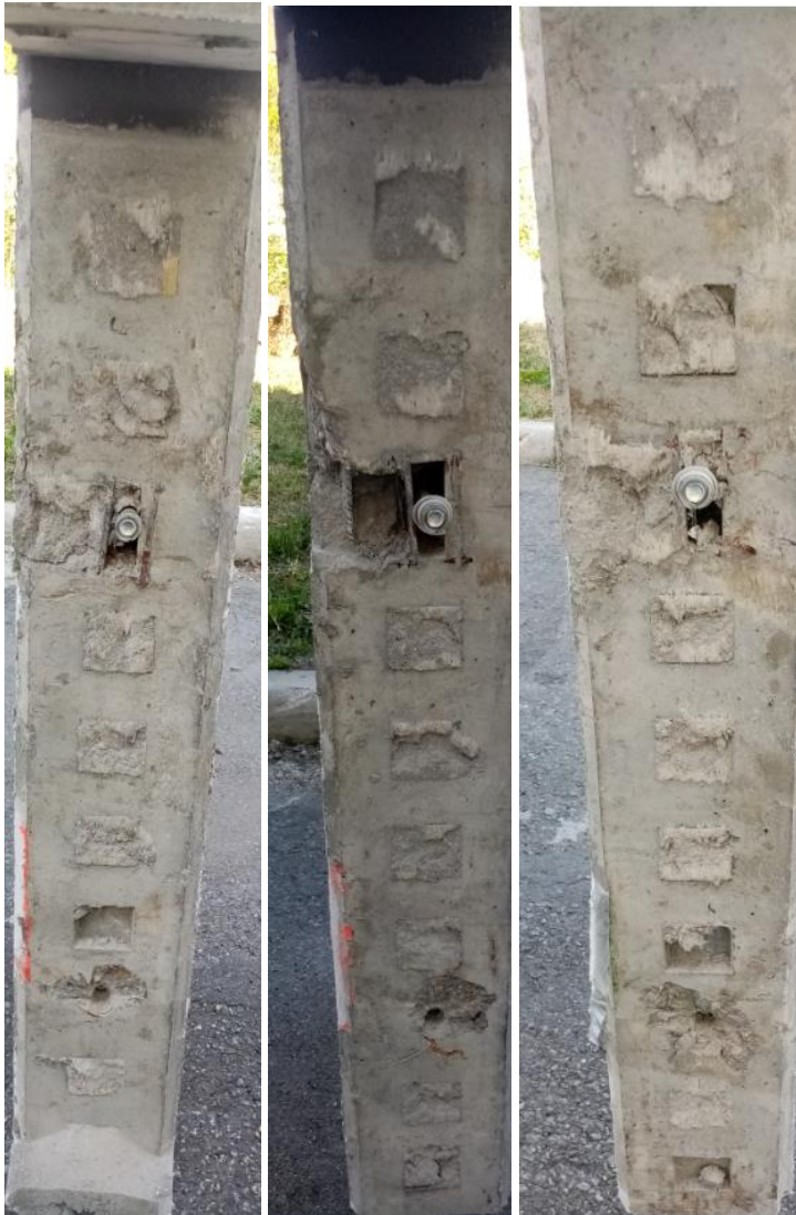
Figure 3-34 Test specimens interfaces after dismantling (from left to right) SA3T1, SA3T2, SA3T3
