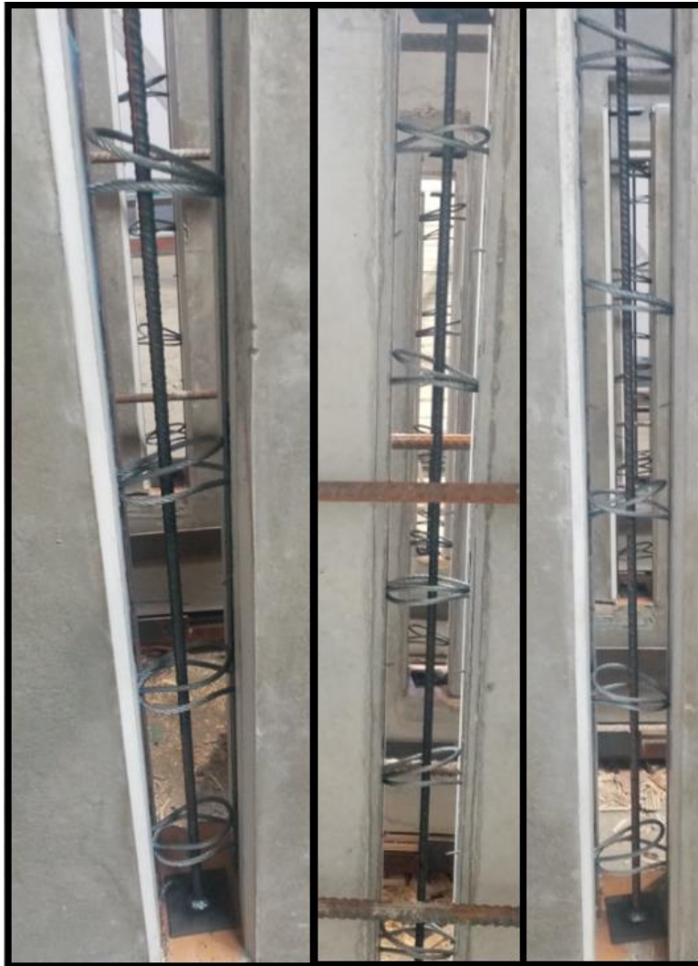
Figure 4-22 Test specimens before joint casting WL3 (from left to right 1st, 2nd and 3rd test specimen)
