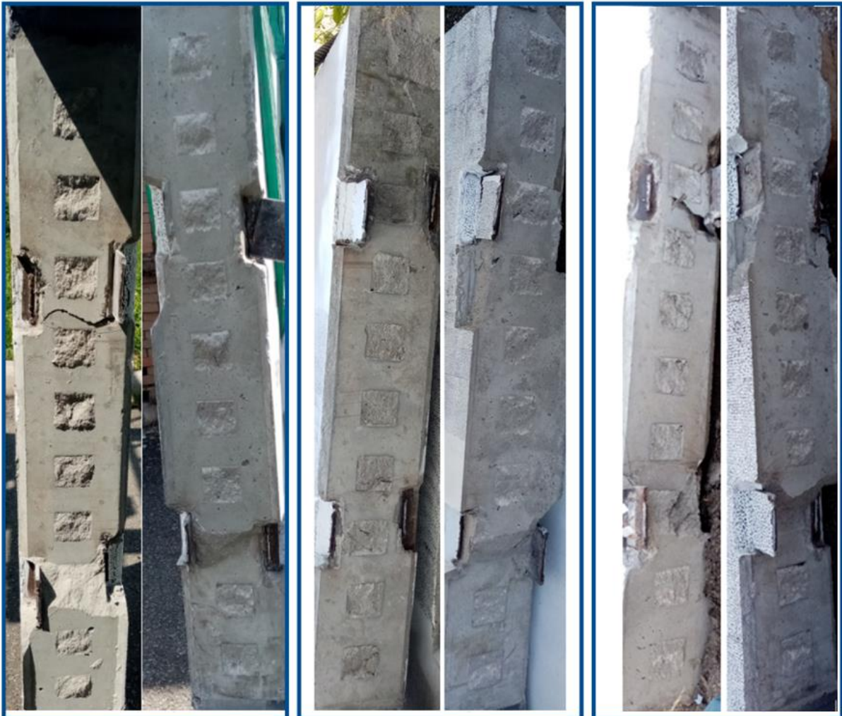
Figure 3-19 Test specimens interfaces after dismantling (from left to right) SA2T1, SA2T2, SA2T3
