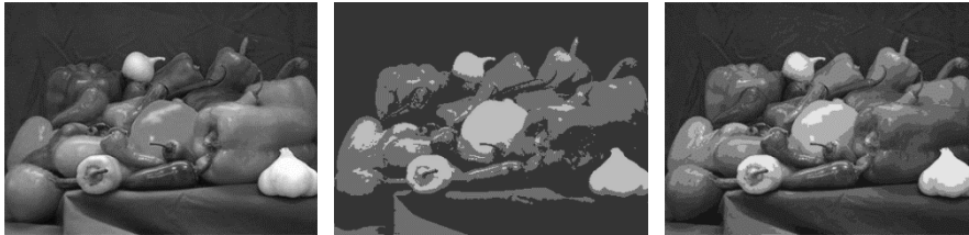
Figure 7.2 – Input grayscale image and its segmentation using K=3 and K=10 centers
