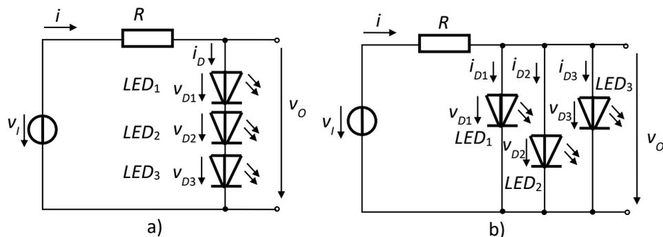
Fig.2.76. Simple circuits with LEDs
