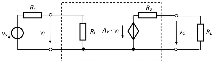
**Fig.3.9.** Amplifier with input voltage source and load resistance
