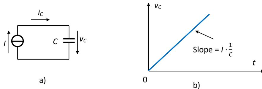
**Fig.1.27.** Charging the capacitor at constant current
