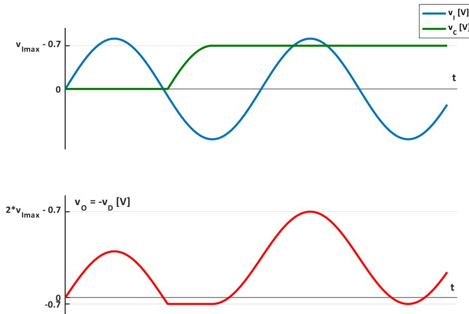
Fig.2.55. Waveforms for  $v_I(t)$ ,  $v_C(t)$  and  $v_O(t)$  for the upward translation circuit
