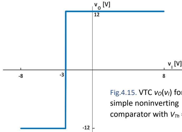
Fig.4.15. VTC  $v_o(v_i)$  for the simple noninverting comparator with  $V_{Th} = -3$  V
