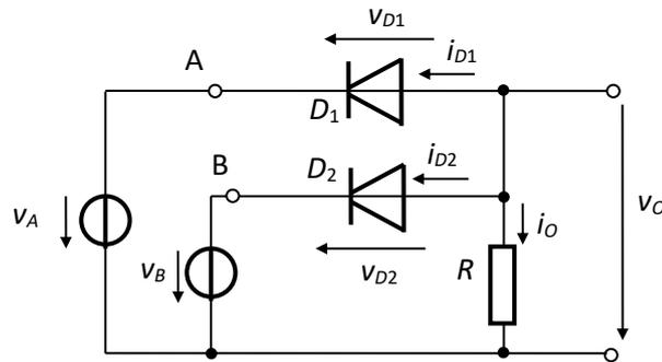
Fig.2.32. Minimum three-port circuit
