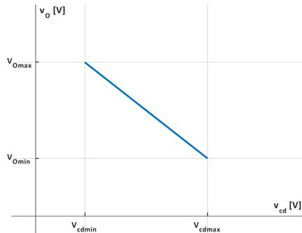
Fig.4.74. VTC  $v_O(v_{cd})$  of an inverting voltage domain converter
