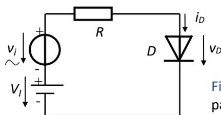
Fig.2.10. Circuit for computing the dynamic parameters of the diode
