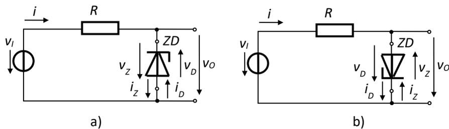
Fig.2.66. Asymmetric double voltage limiters with ZD
