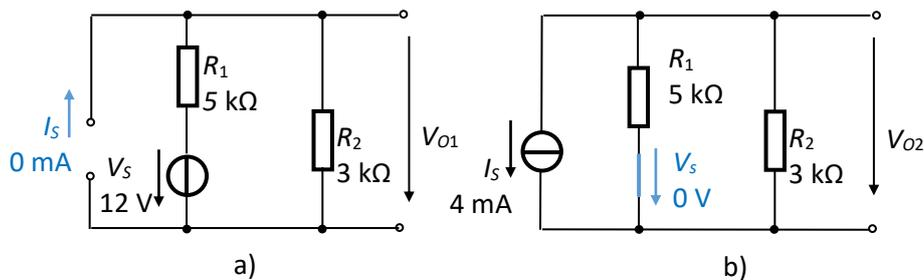
Fig.1.16. Equivalent circuits for applying the superposition method
