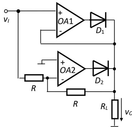
Fig.4.88. Fullwave active rectifier with superdiodes
