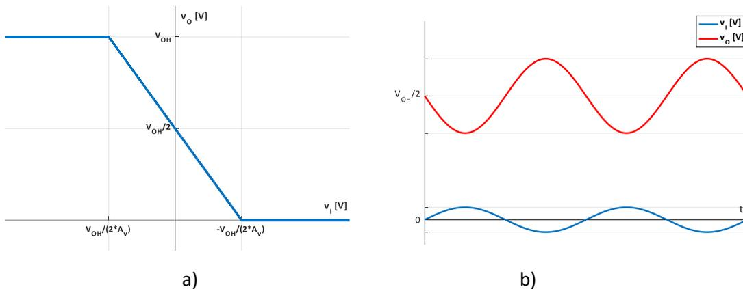
Fig.4.85. Inverting amplifier with unipolar supply
