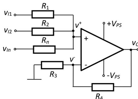
Fig.4.57. Noninverting summing amplifier with  $n$  input voltages
