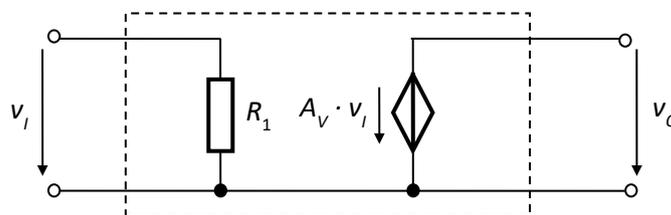
Fig.4.45. Modelling the inverting amplifier as a VCVS
