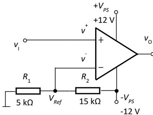
Fig.4.14. Simple noninverting comparator with negative threshold voltage
