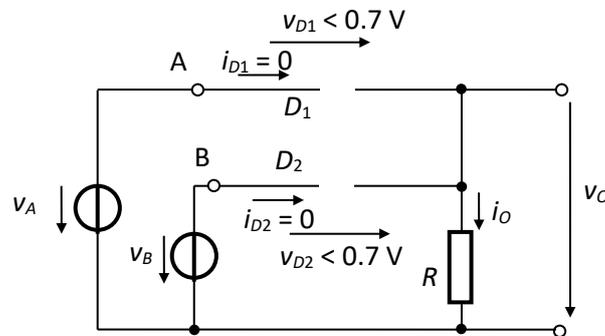
Fig.2.29. Equivalent circuit –  $D_1$  and  $D_2$  off
