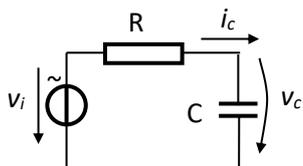
Fig.1.28. RC series circuit with ac voltage source
