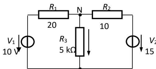
Fig.1.20. Illustration of Millman’s theorem - example
