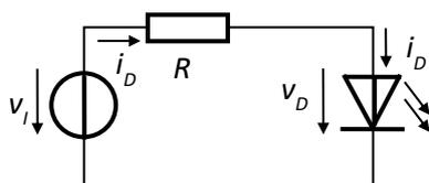
Fig.2.75. Simple circuit with LED and  $R$
