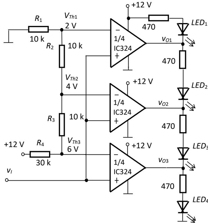
Fig.4.19. Optical voltage level indicator –one LED is *on* at any given time
