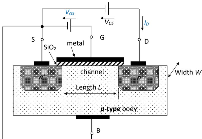
Fig.5.17. NMOS - simplified physical structure with voltage sources
