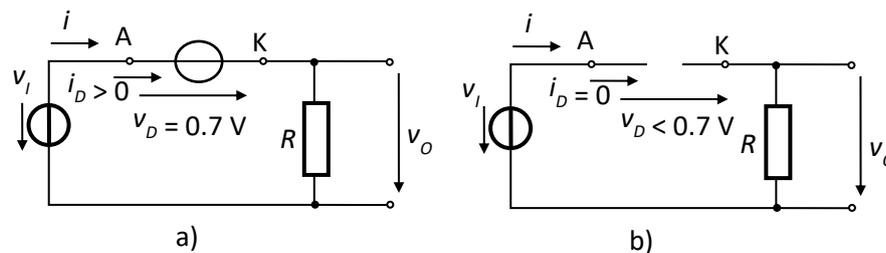
**Fig.2.19.** Equivalent schematic for the circuit in Fig.2.18. a)
