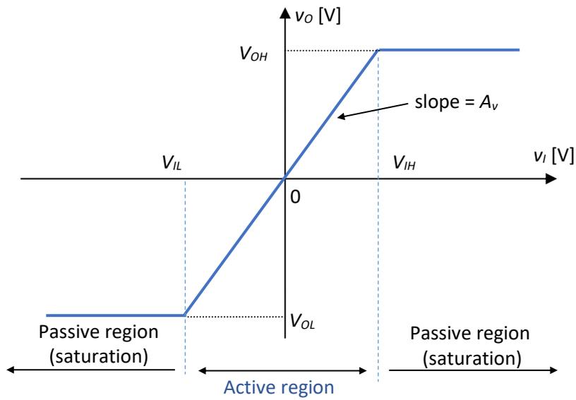
Fig.3.11. VTC  $v_o(v_i)$  for the voltage amplifier with differential supply
