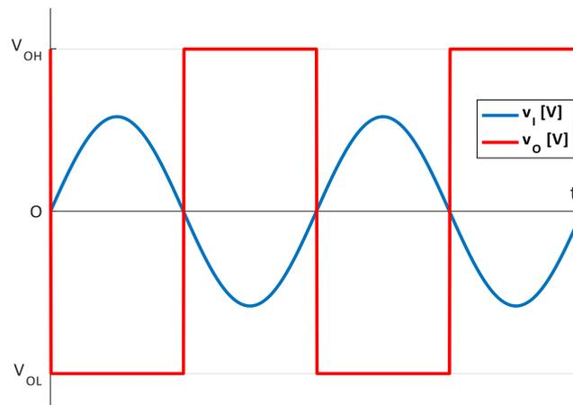
Fig.4.9. Simple inverting comparator - waveforms for  $v_i(t)$  and  $v_o(t)$
