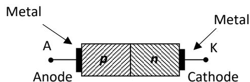
Fig.2.1. Simplified physical structure of the  $pn$  junction
