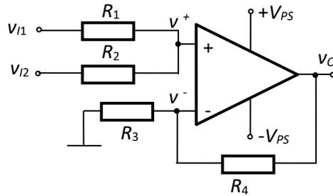
Fig.4.56. Noninverting summing amplifier with two input voltages
