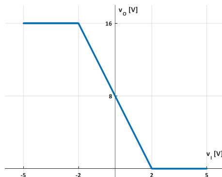
Fig.4.86. VTC  $v_O(v_I)$
