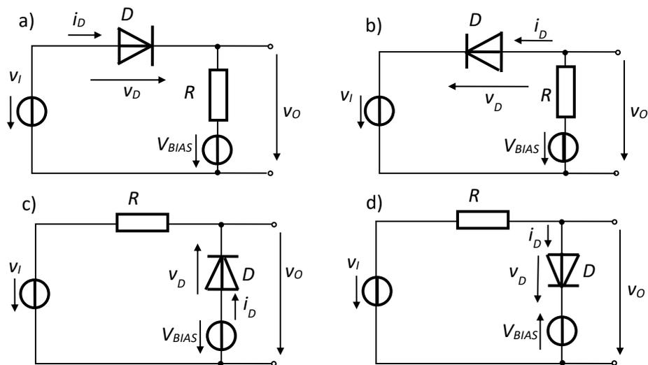
**Fig.2.37. DR voltage limiters with  $V_{BIAS}$**
