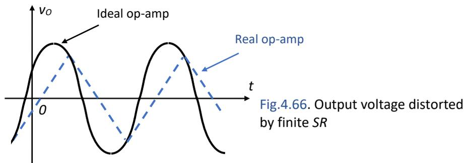
Fig.4.66. Output voltage distorted by finite SR
