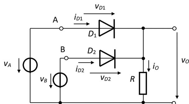
Fig.2.28. Maximum three-port circuit
