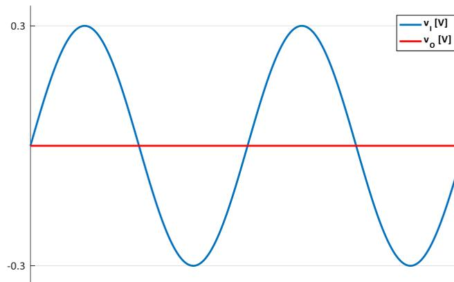
Fig.2.23. Waveforms of  $v_i(t)$  and  $v_o(t)$  for  $v_i(t) = 0.3\sin\omega t$  [V]
