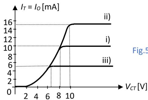
Fig.5.7. Transfer characteristics  $I_T(V_{CT})$  for the circuit in Fig.5.4
