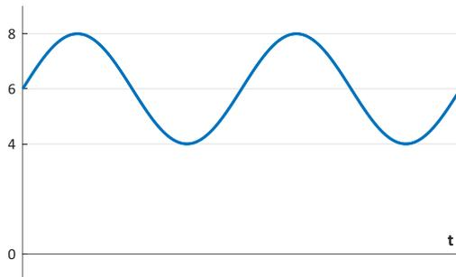
Fig.1.2. Graphical representation of  $v_s(t) = 6 + 2\sin\omega t$  [V]
