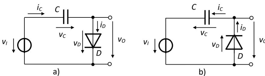
Fig.2.54. *DC* switching circuits with the output on D
