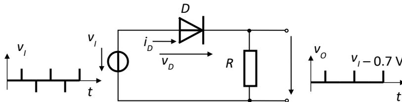
Fig.2.45. Positive pulses selector circuit
