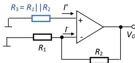
Fig.4.70. Op-amp with negative feedback and bias currents
