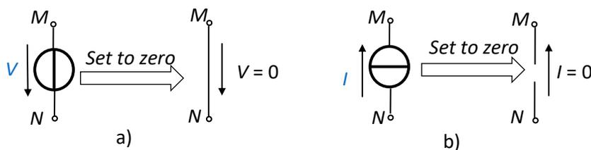
Fig.1.14. Sources set to zero (passive)
