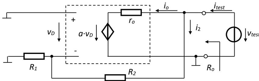
Fig.4.68. Determining the output resistance of the noninverting amplifier
