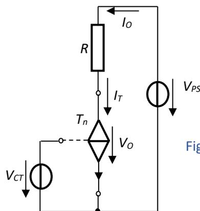
Fig.5.4.  $T_n$  in a circuit with series voltage supply
