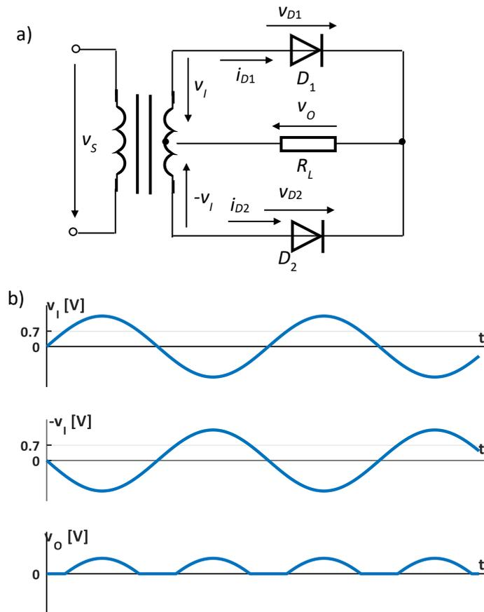
Fig.2.47. Full-wave rectifier obtained with a DR spatial maximum multi-port
