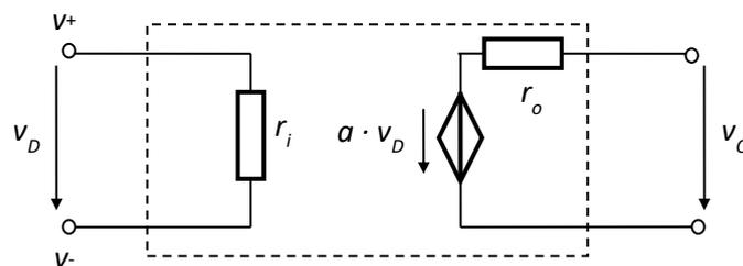
Fig.4.4. Modeling the op-amp with a voltage-controlled voltage source
