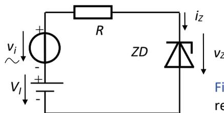
Fig.2.65. Circuit for computing the relative regulation factor of ZD
