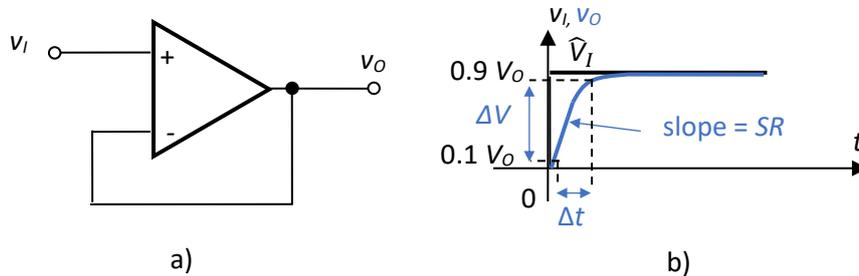
Fig.4.65. Noninverting voltage follower with step input voltage
