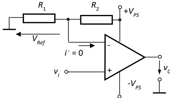
**Fig.4.12.** Simple comparator, noninverting,  $V_{Th} \neq 0$  V, with resistive divider
