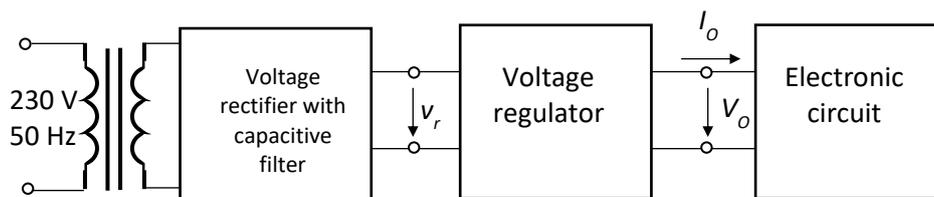
Fig.2.58. Block diagram of a dc power supply
