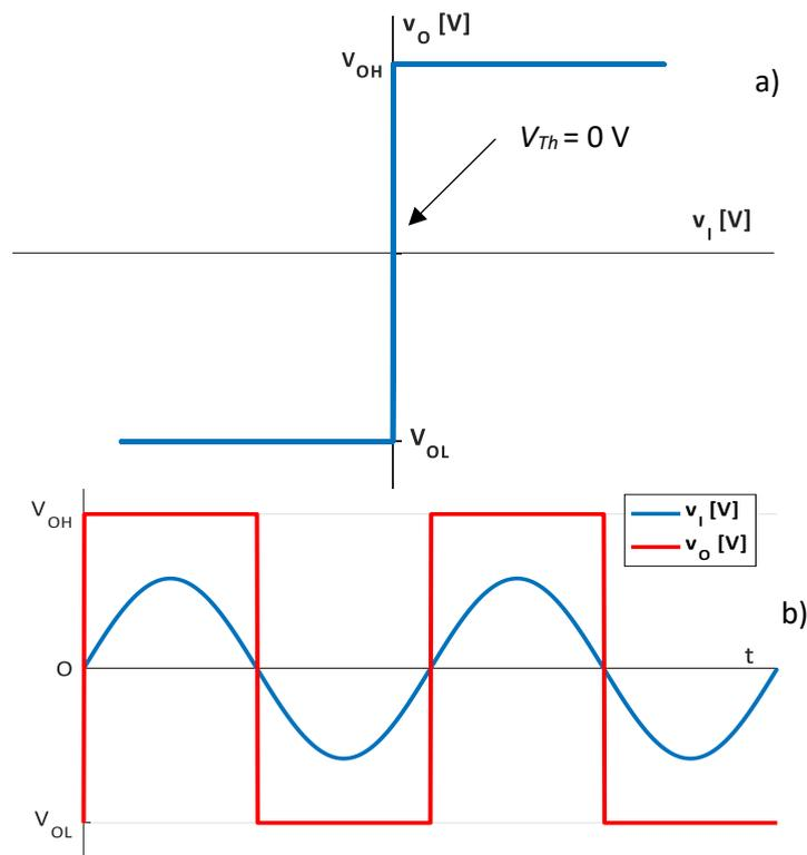
**Fig.4.7.** Simple comparator, noninverting,  $V_{th} = 0 \text{ V}$
