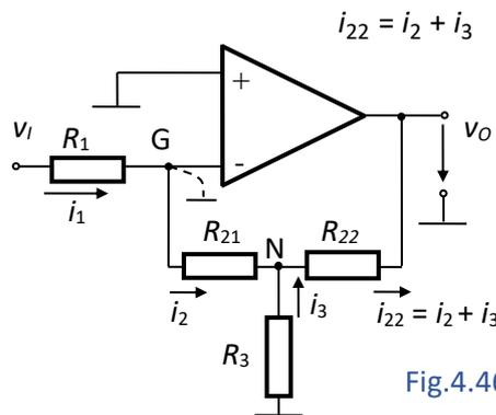
Fig.4.46. T-network inverting amplifier
