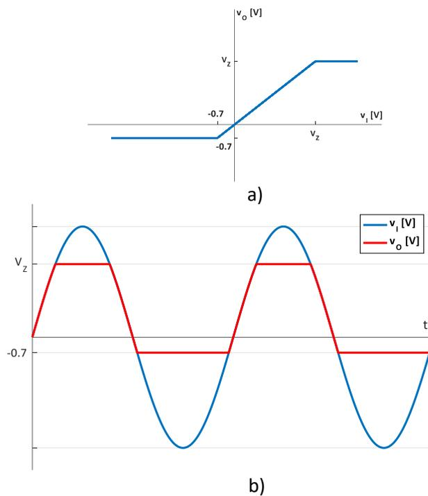
Fig.2.68. Asymmetric double voltage limiter a) VTC  $v_O(v_I)$ ; b) waveforms.
