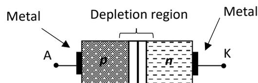
Fig.2.2. The  $pn$  junction with no applied voltage
