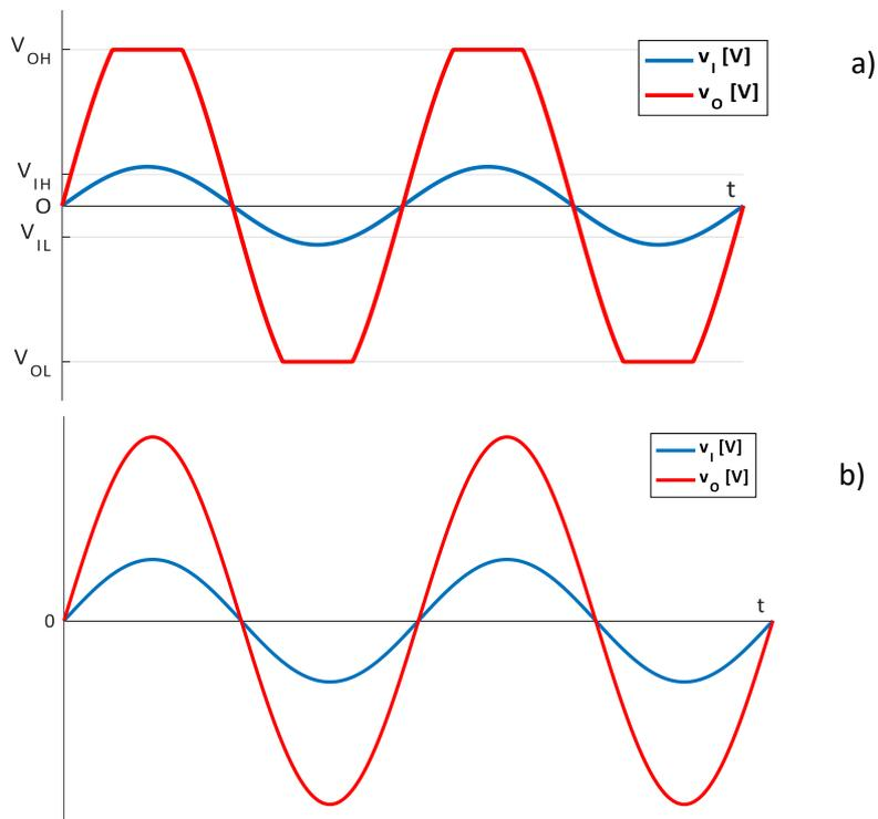
Fig.3.12. Waveforms for  $v_i(t)$  and  $v_o(t)$  for the voltage amplifier with differential supply
