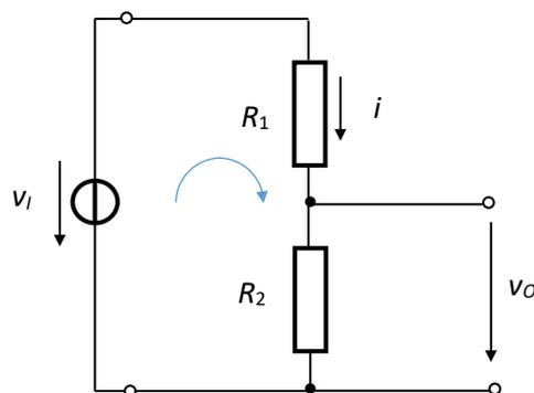
Fig.1.10. Voltage divider
