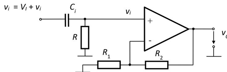
Fig.4.77. Noninverting amplifier with capacitive coupling
