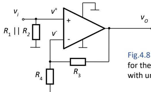
**Fig.4.81.** Equivalent ac circuit for the noninverting amplifier with unipolar supply
