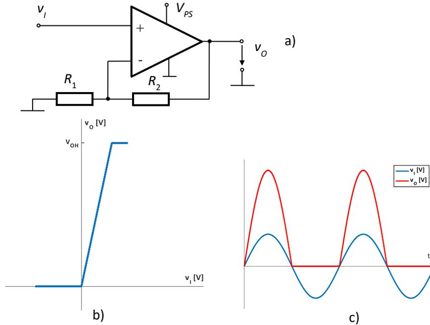
**Fig.4.78.** Noninverting amplifier with unipolar supply
