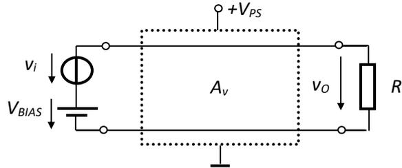
Fig.3.13. Voltage amplifier with unipolar supply and  $V_{BIAS}$
