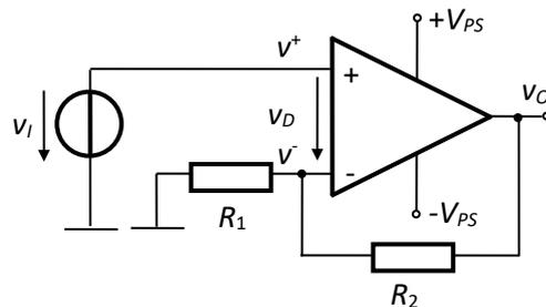
Fig.4.36. Noninverting voltage amplifier with op-amp
