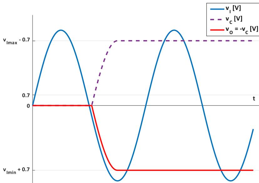
Fig.2.53. Waveforms for the negative peak detector
