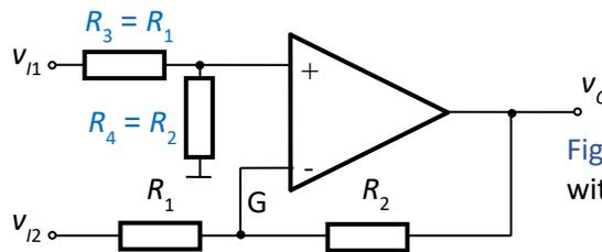
Fig.4.60. Differential amplifier with resistive divider
