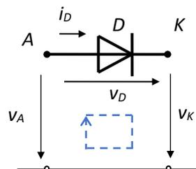
Fig.2.26. Voltage drop across the diode  $v_D$  expressed as the difference between  $v_A$  and  $v_K$
