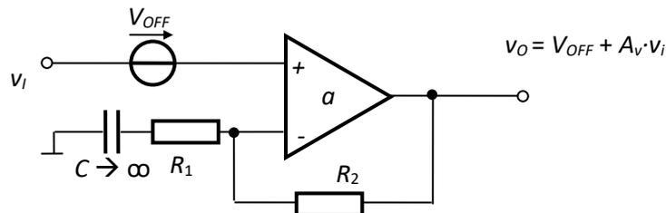
Fig.4.69. Capacitive coupling of the negative feedback loop to reduce the effect of the offset voltage
