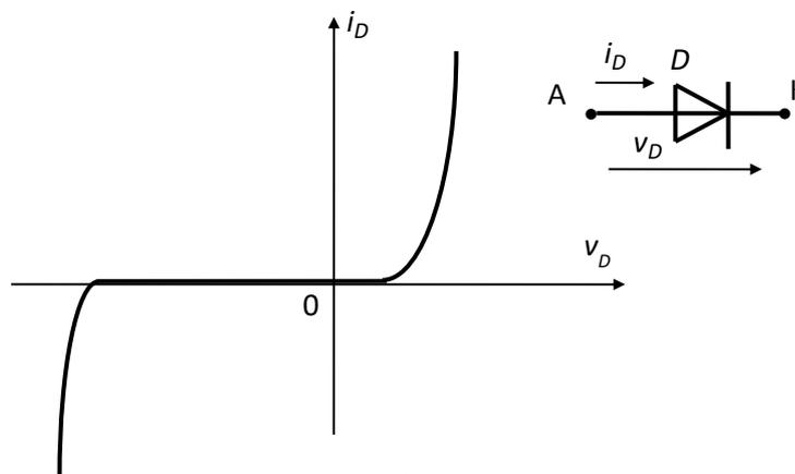
Fig.2.5.  $i_D(v_D)$  characteristic of a silicon diode
