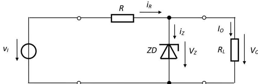
Fig.2.71. Parametric voltage regulator with ZD
