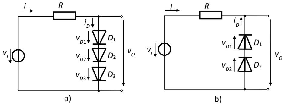
**Fig.2.35** Voltage limiters with multiple diodes in series
