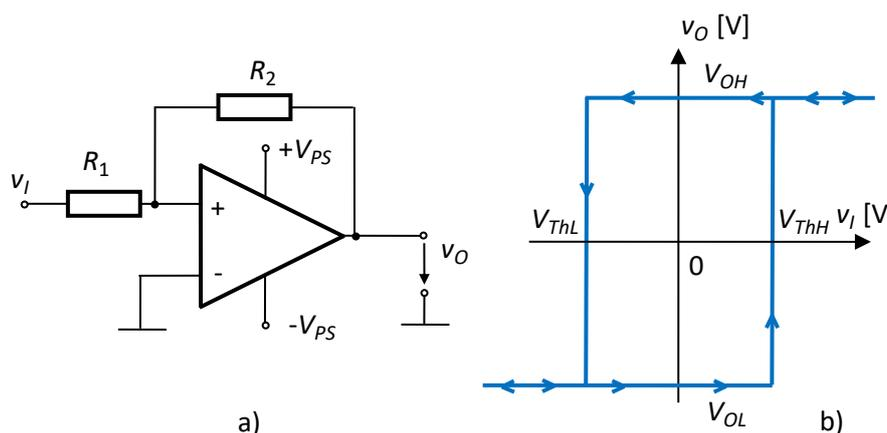
Fig.4.25. Noninverting hysteresis comparator with symmetric thresholds
