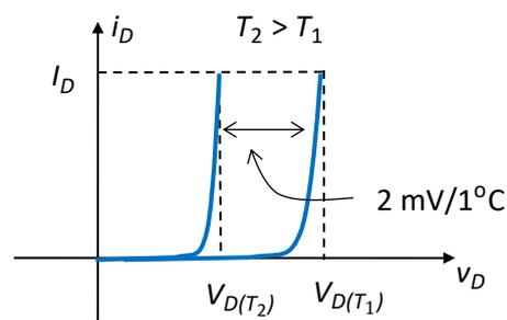
Fig.2.7.  $i_D(v_D)$  characteristic of the  $pn$  junction for different temperatures
