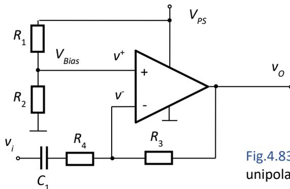
Fig.4.83. Inverting amplifier with unipolar supply – final circuit
