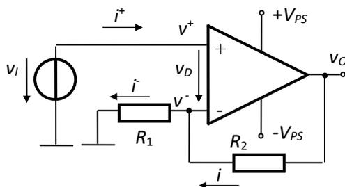
**Fig.4.37.** Noninverting amplifier
