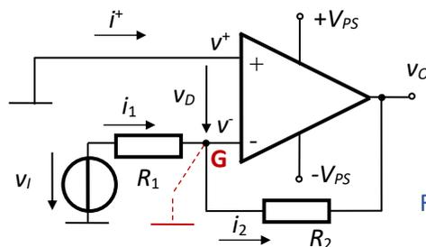
Fig.4.43. Inverting amplifier
