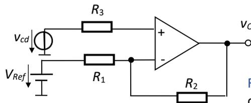
Fig.4.71. Noninverting voltage domain converter
