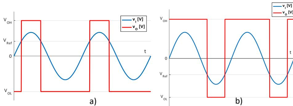
**Fig.4.18.** Waveforms for  $v_i(t)$  and  $v_o(t)$  for the circuit in Fig.4.17
