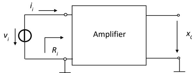
Fig.3.4. Circuit for computing  $R_i$
