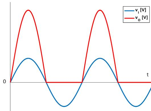
Fig.3.15. Waveforms of  $v_i(t)$  and  $v_o(t)$  for the voltage amplifier with unipolar supply in the active region
