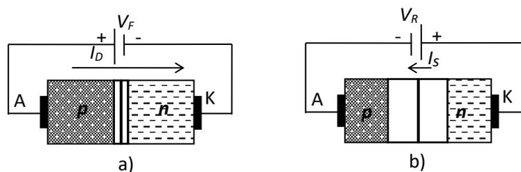
Fig.2.3. The  $pn$  junction in a) forward biasing; b) reverse biasing.
