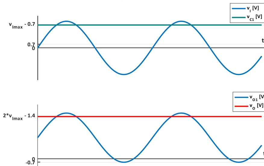
Fig.2.57. Steady-state waveforms for  $v_i(t)$ ,  $v_{C1}(t)$ ,  $v_{O1}(t)$  and  $v_O(t)$  for the positive voltage doubler in Fig.2.56. b)
