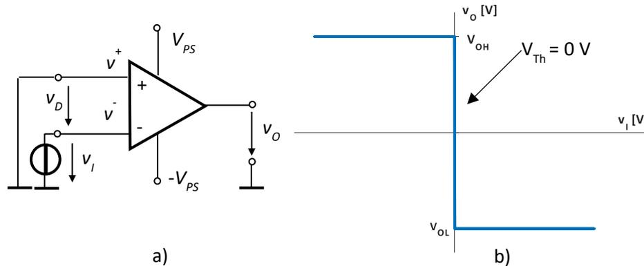
Fig.4.8. Simple inverting comparator with with  $V_{Th} = 0 \text{ V}$ : a) circuit;) VTC  $v_o(v_i)$ .
