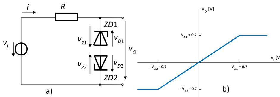
Fig.2.69. Symmetrical voltage limiter a) circuit; b) VTC  $v_O(v_I)$ .
