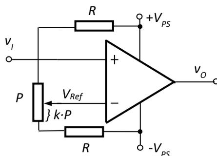
**Fig.4.17.** Circuit for obtaining a square wave from a sinusoidal wave
