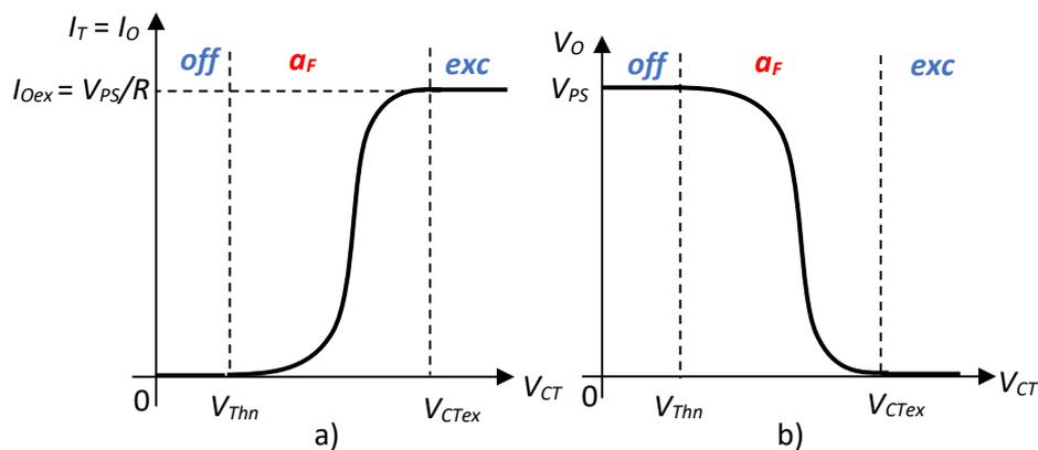
Fig.5.5. Transfer characteristics
