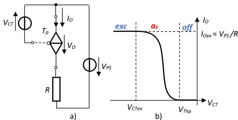
Fig.5.6.  $P$ -type transistor  $T_p$
