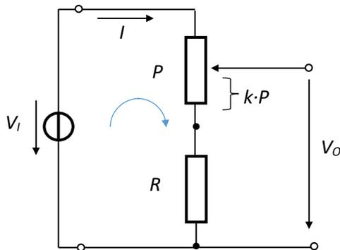
Fig.1.12. Final circuit for the adjustable voltage divider with  $R$  and  $P$
