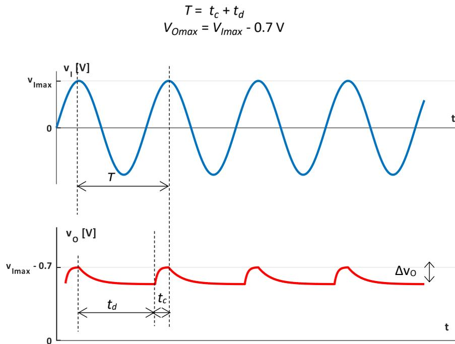
Fig.2.61. DRC rectifier waveforms
