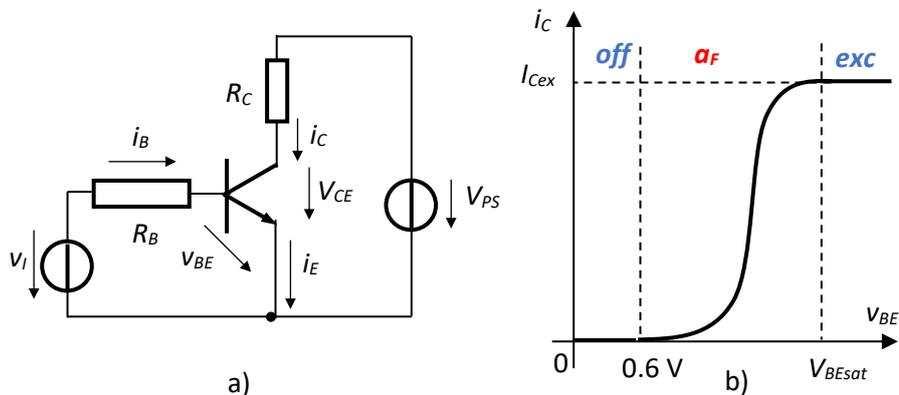
**Fig.5.12.** Circuit with BJT to determine the static transfer characteristic
