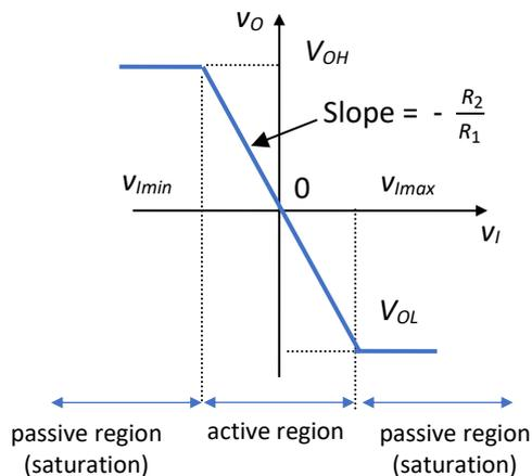
Fig.4.38. VTC  $v_O(v_I)$  for the inverting amplifier
