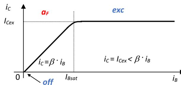
Fig.5.14. Current transfer characteristic  $i_C(i_B)$  for the *npn* BJT
