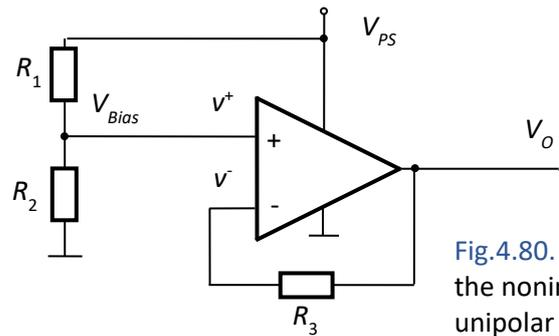
**Fig.4.80.** Equivalent dc circuit for the noninverting amplifier with unipolar supply
