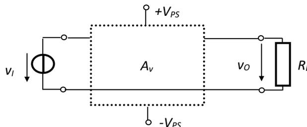
Fig.3.10. Voltage amplifier with differential supply
