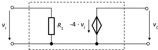
Fig.4.53. Model of the inverting amplifier
