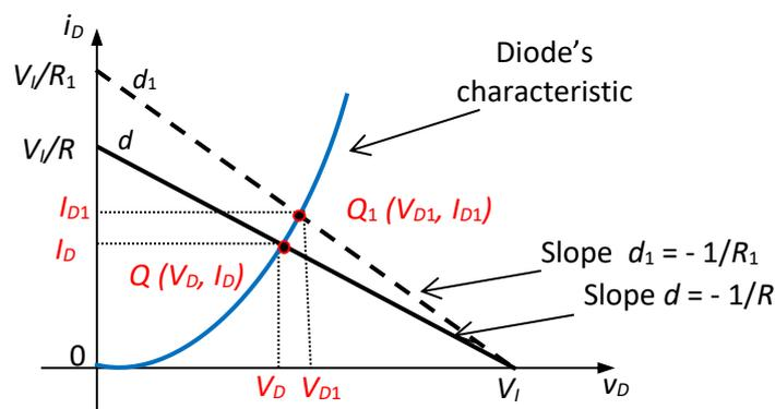
Fig.2.9. Graphical method for solving a simple *DR* circuit
