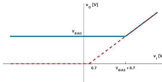
**Fig.2.38. VTC  $v_O(v_I)$  for the inferior voltage limiter in Fig.2.37. a)**
