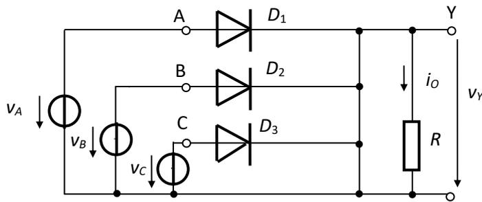
Fig.2.50. Three input OR logic circuit
