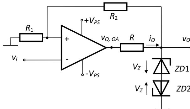
Fig.4.34. Inverting hysteresis comparator with output voltage independent of the two power supplies
