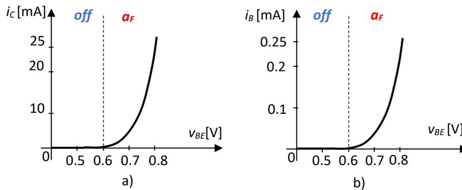
Fig.5.13. Static characteristics for the *npn* BJT
