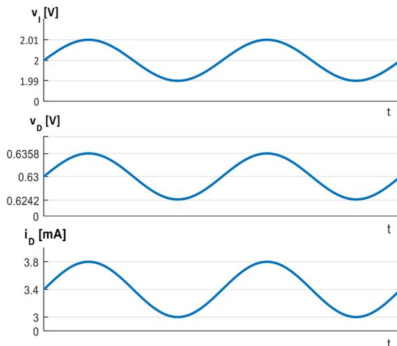
Fig.2.15. Waveforms of  $v_i(t)$ ,  $v_D(t)$  and  $i_D(t)$
