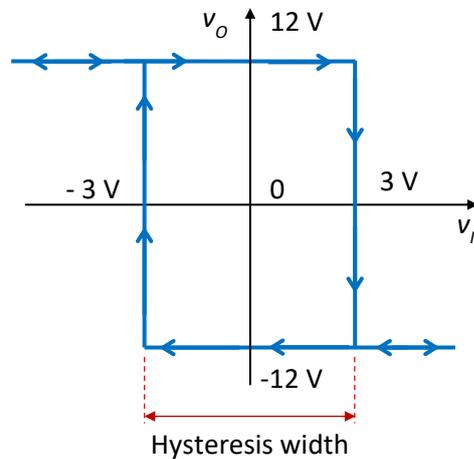
Fig.4.29. VTC  $v_o(v_i)$
