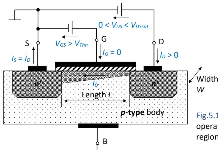
Fig.5.19. NMOS operation in the linear region
