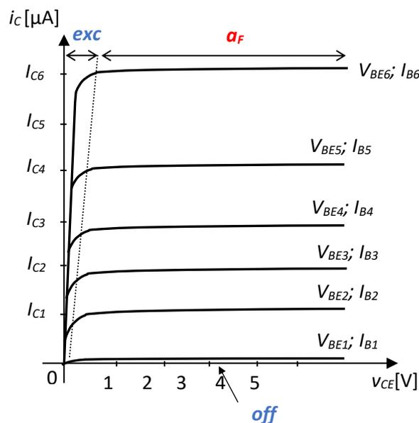
Fig.5.15. Family of output characteristics  $i_c(v_{CE})$  for the *npn* BJT
