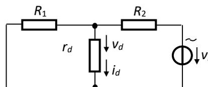
Fig.2.14. The ac equivalent circuit (small-signal)
