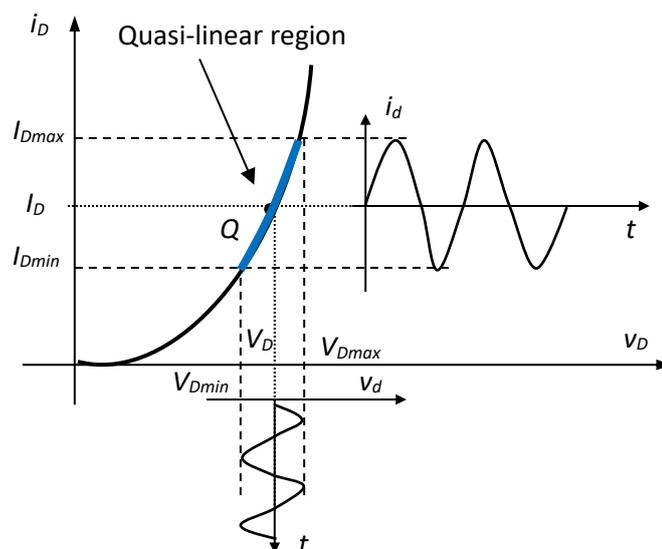
Fig.2.11. Superposition of variable signals on dc signals in the quasi-linear region around the quiescent point on the characteristic of a diode
