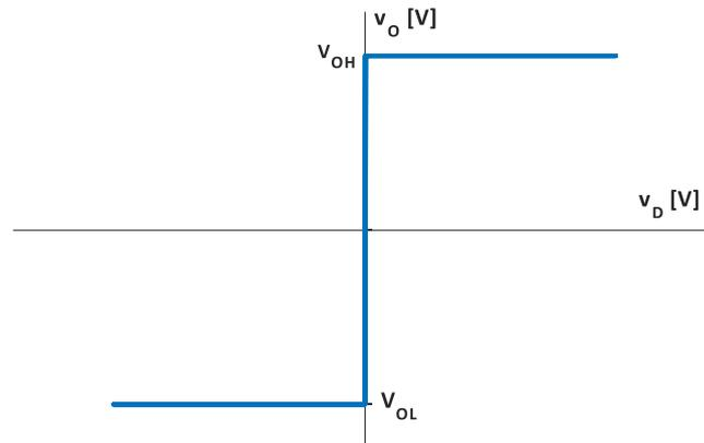
Fig.4.5. VTC  $v_o(v_D)$  of an ideal op-amp
