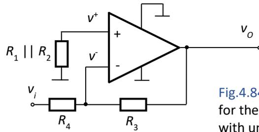
Fig.4.84. Equivalent ac circuit for the inverting amplifier with unipolar supply
