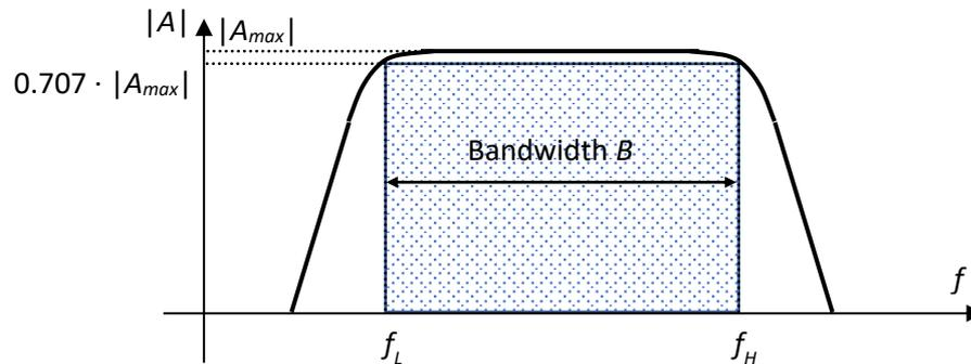
Fig.3.6. Gain-frequency plot of an amplifier
