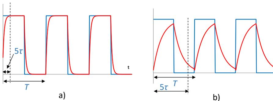
Fig.1.29. Voltage across a capacitor in ac
