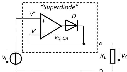
Fig.4.87. Positive halfwave active rectifier with superdiode
