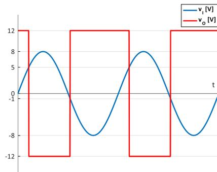
Fig.4.31. Waveforms of  $v_i(t)$  and  $v_o(t)$
