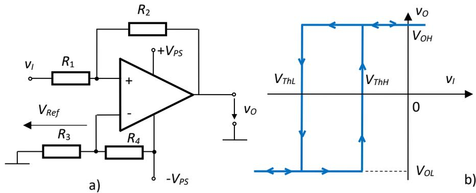
Fig.4.28. Noninverting hysteresis comparator with asymmetric thresholds
