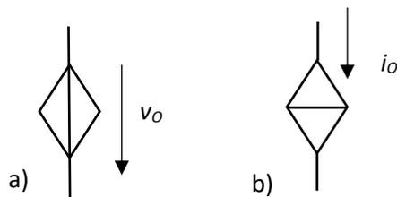
Fig.3.7. Symbols for controlled sources
