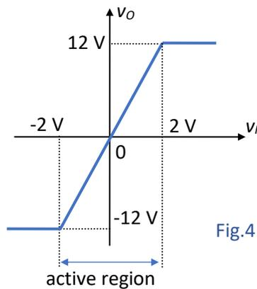
Fig.4.49. VTC  $v_o(v_i)$  for the noninverting amplifier
