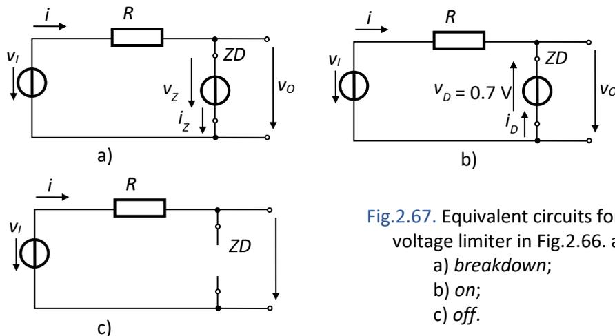
Fig.2.67. Equivalent circuits for the voltage limiter in Fig.2.66. a) *breakdown*;
