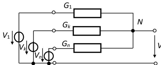
Fig.1.19. Illustration of Millman’s theorem
