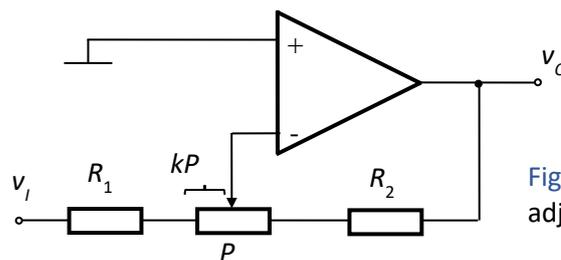
Fig.4.48. Inverting amplifier with adjustable gain
