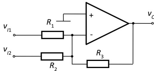
Fig.4.58. Inverting summing amplifier with two input voltages
