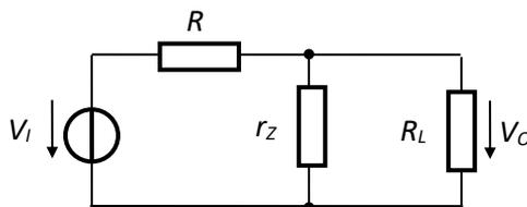
Fig.2.72. Parametric voltage regulator with ZD:
