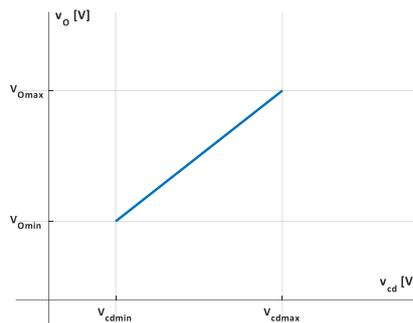
Fig.4.72. VTC  $v_O(v_{cd})$  of a noninverting voltage domain converter
