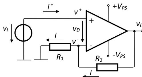
Fig.4.63. Noninverting amplifier
