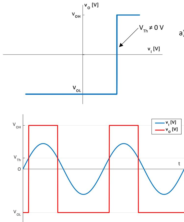
**Fig.4.11.** Simple comparator, noninverting,  $V_{Th} \neq 0$  V
