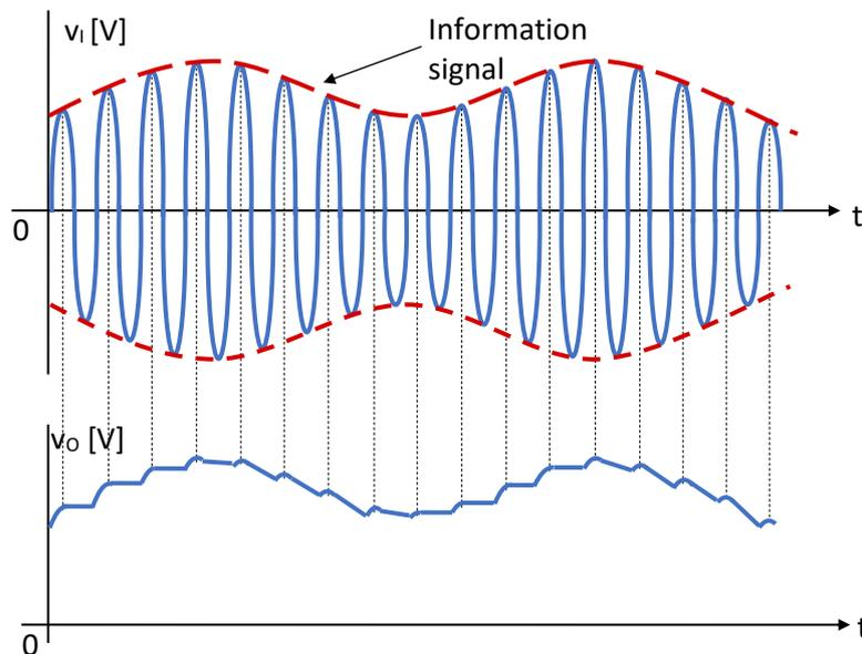
Fig.2.62. Envelope detection of the carrier signal [2]
