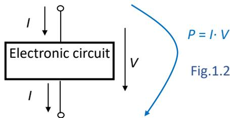
Fig.1.21. Current, voltage, power for an electronic circuit
