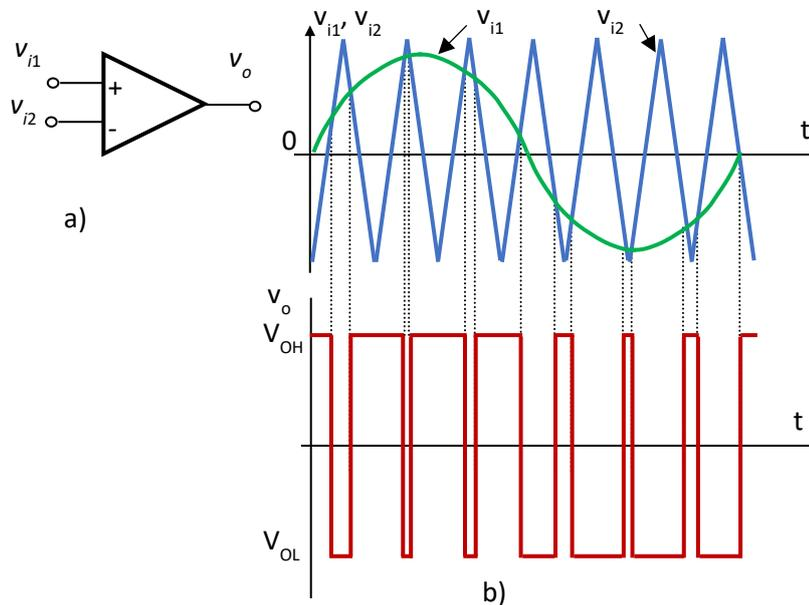
**Fig.4.21.** Pulse width modulation
