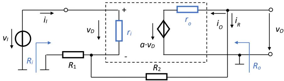
Fig.4.67. Model of the noninverting amplifier
