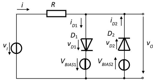
Fig.2.44. Double voltage limiter
