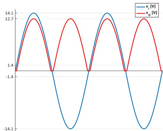
Fig.2.49. Waveforms for the full-wave diode bridge rectifier
