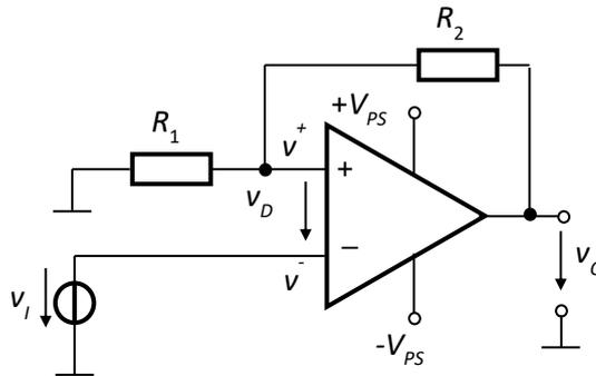
Fig.4.23. Hysteresis comparator, inverting, with symmetric threshold voltages
