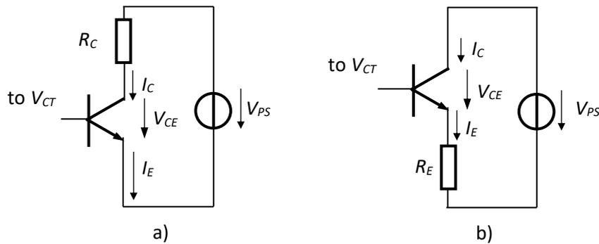
**Fig.5.11.** Limiting the controlled current through the BJT
