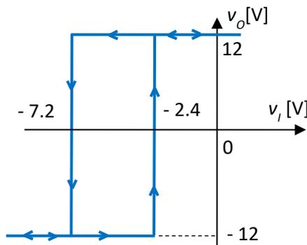
Fig.4.32. VTC  $v_o(v_i)$
