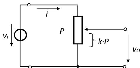
Fig.1.11. Adjustable voltage divider
