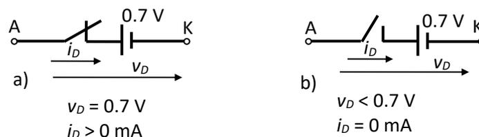
Fig.2.17. Constant voltage drop model of the diode,  $v_D = 0.7\text{ V}$
