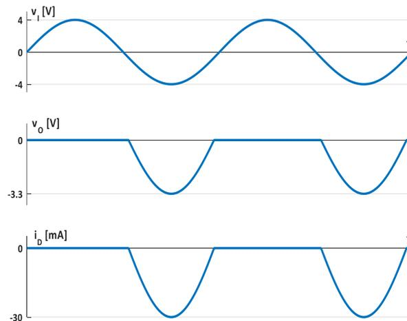
Fig.2.25. Waveforms for  $v_I(t)$ ,  $v_O(t)$  and  $i_D(t)$  for  $v_I(t) = 4\sin\omega t$  [V]
