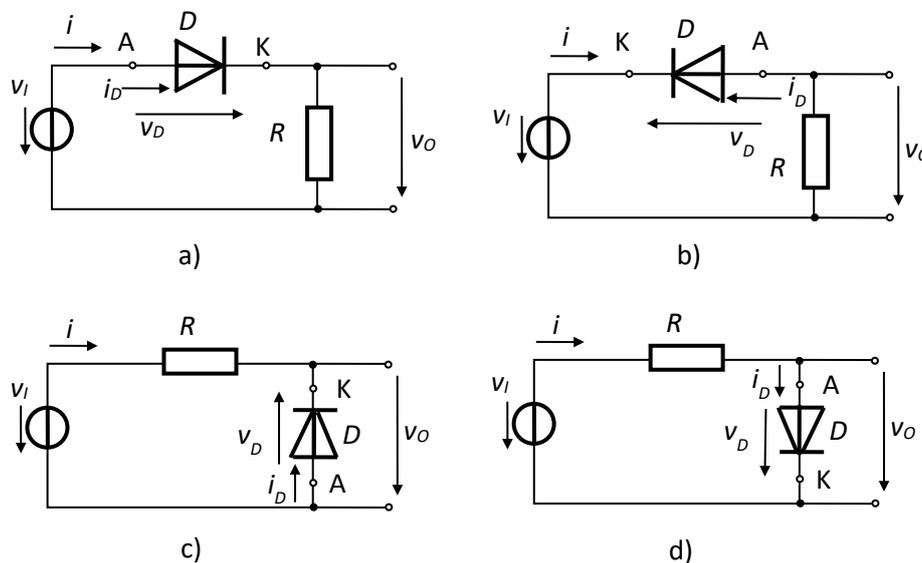
Fig.2.18. Two-port DR series circuits
