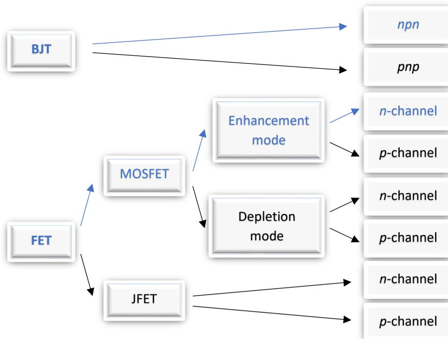
Fig.5.1. Types of transistors
