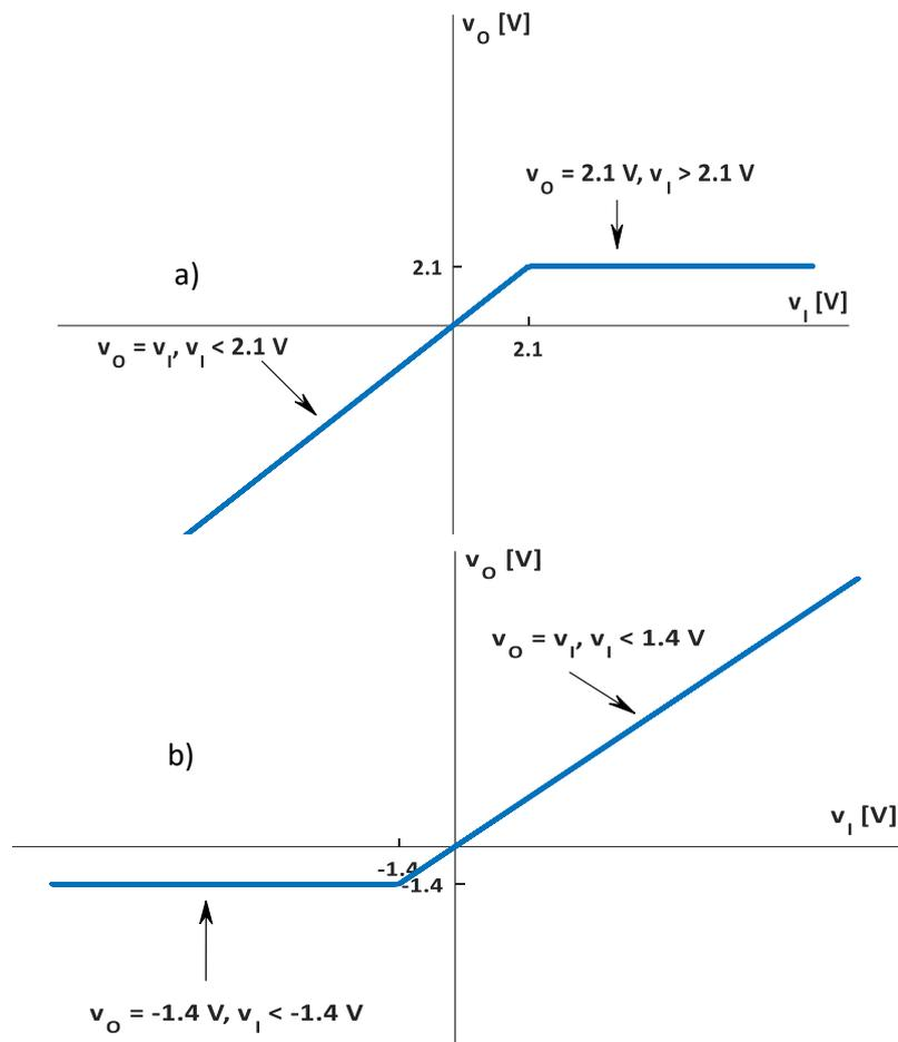
**Fig.2.36.** VTC  $v_o(v_i)$  for the circuits in Fig.2.35.
