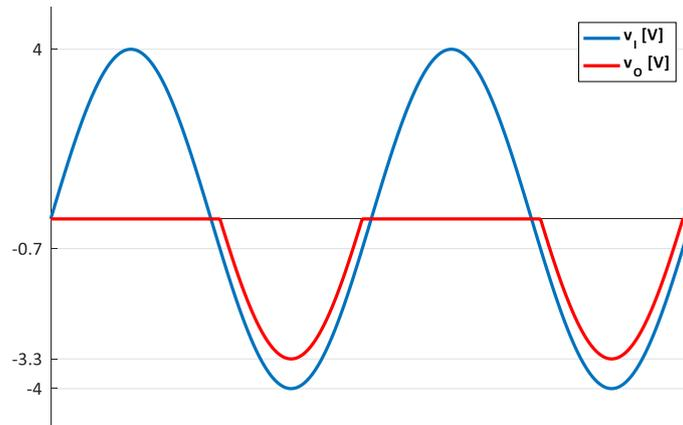
Fig.2.24. Waveforms of  $v_i(t)$  and  $v_o(t)$  for  $v_i(t) = 4\sin\omega t$  [V]
