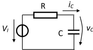
Fig.1.25. RC series circuit with a dc voltage source
