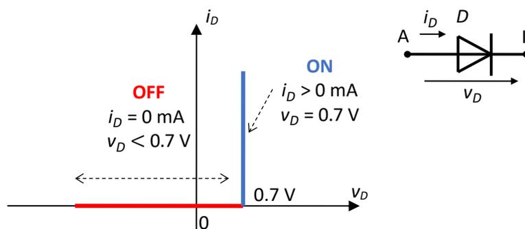
Fig.2.16. The  $i_D(v_D)$  characteristic for the constant voltage drop model of the diode,  $v_D = 0.7\text{ V}$
