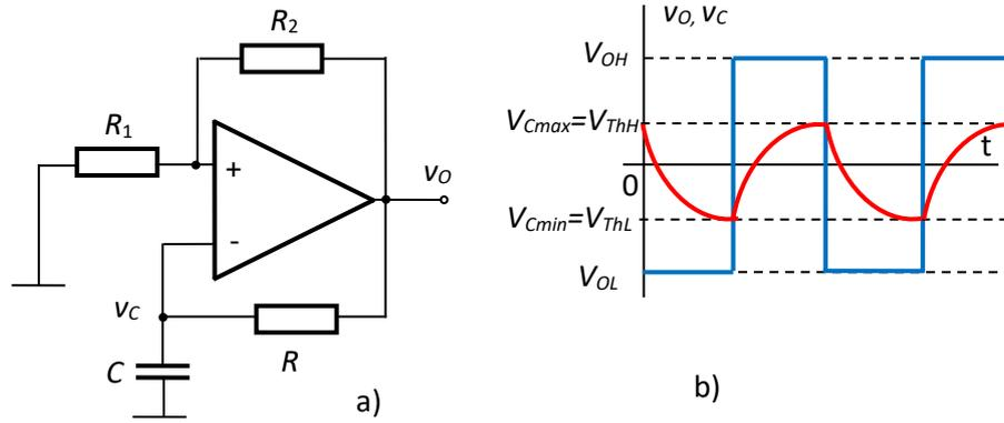
Fig.4.35. RC and positive feedback op-amp oscillator
