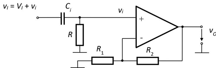
Fig.4.42. Noninverting amplifier with capacitive coupling
