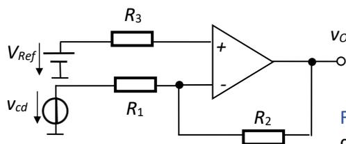
Fig.4.73. Inverting voltage domain converter
