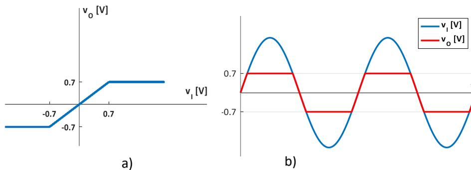
Fig.2.43. Double voltage limiter a) VTC  $v_o(v_i)$ ; b) waveforms.
