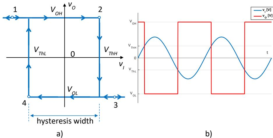
Fig.4.24. Hysteresis comparator, inverting, with symmetric threshold voltages
