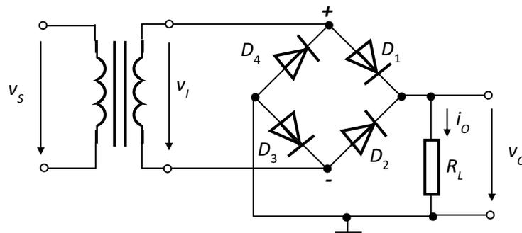
Fig.2.48. Full-wave diode bridge rectifier
