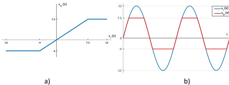
**Fig.2.70.** Asymmetric double voltage limiter with  $V_{Omax} = 7.5 \text{ V}$  and  $V_{Omin} = -4 \text{ V}$
