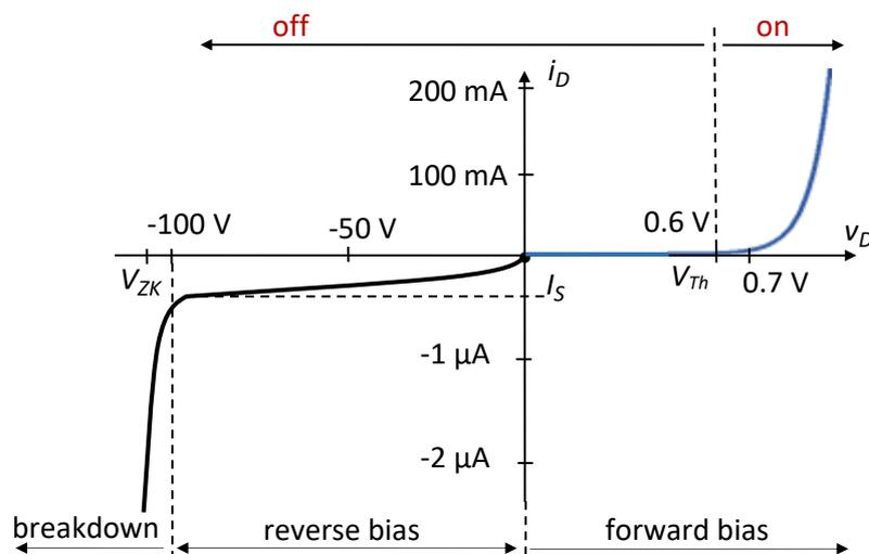
Fig.2.6.  $i_D(v_D)$  characteristic of a silicon diode with expanded negative current scale and compressed negative voltage scale.
