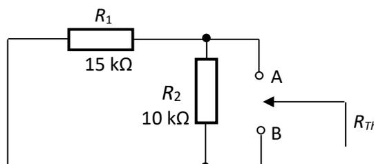
Fig.1.18. Equivalent circuit for computing  $R_{Th}$
