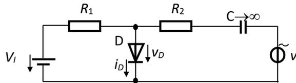
Fig.2.12. Circuit for computing the parameters of the diode
