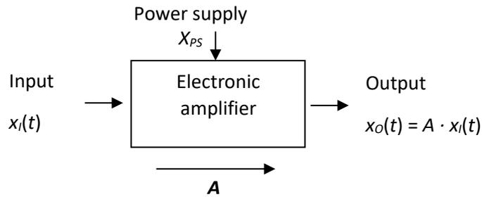
Fig.3.1. “Black-box” representation of the electronic amplifier
