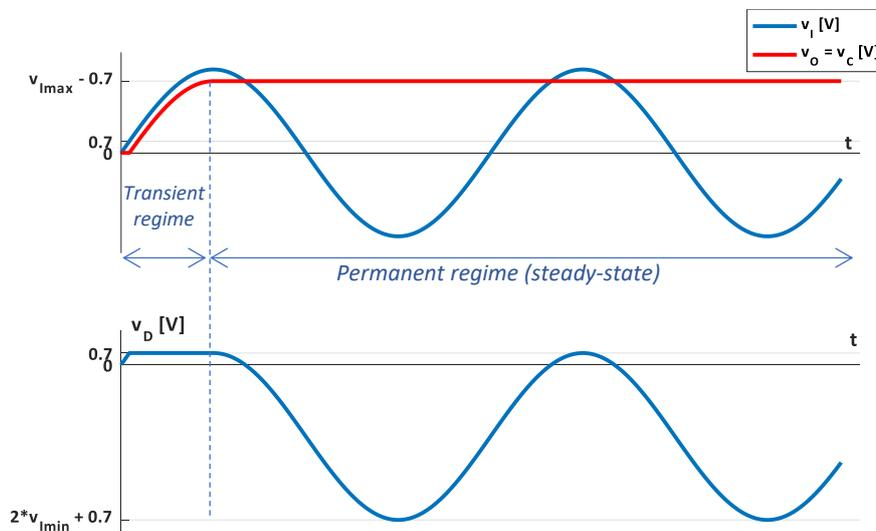
Fig.2.52. Waveforms for the positive peak detector
