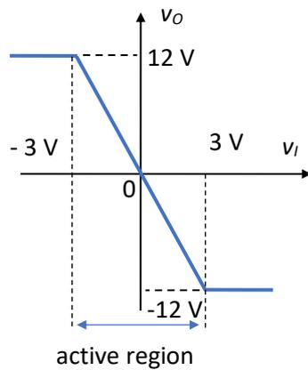
Fig.4.52. VTC  $v_o(v_i)$  for the inverting amplifier
