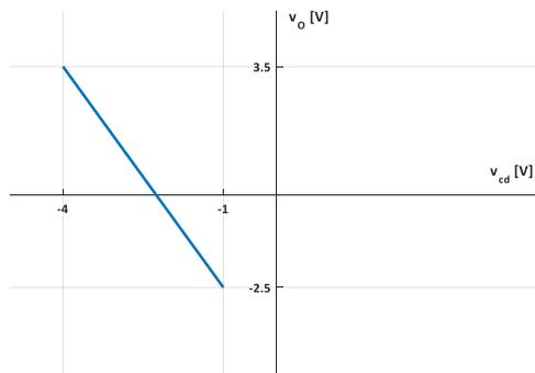
Fig.4.76. VTC  $v_O(v_{cd})$  for the proposed inverting voltage domain converter
