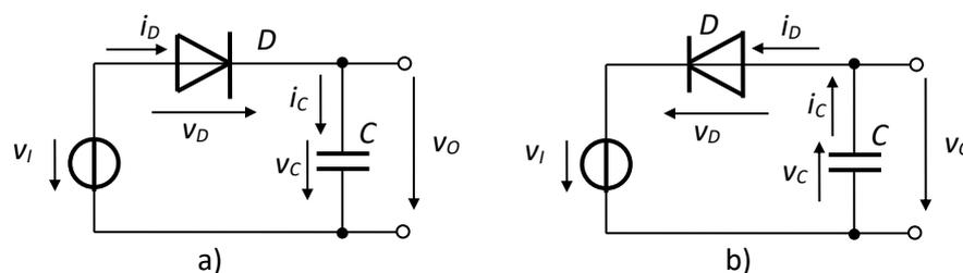
**Fig.2.51.** DC circuits, output on C
