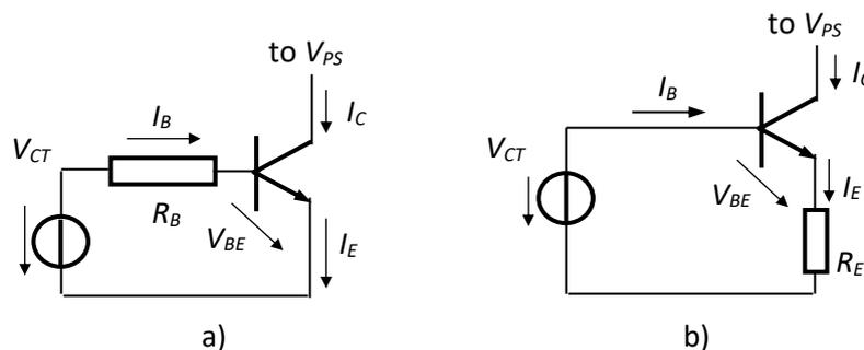
Fig.5.10. Limiting the control current through the BJT
