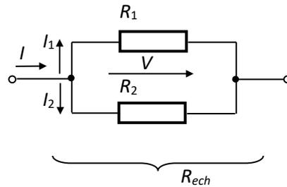
Fig.1.9. Parallel connection of two resistors
