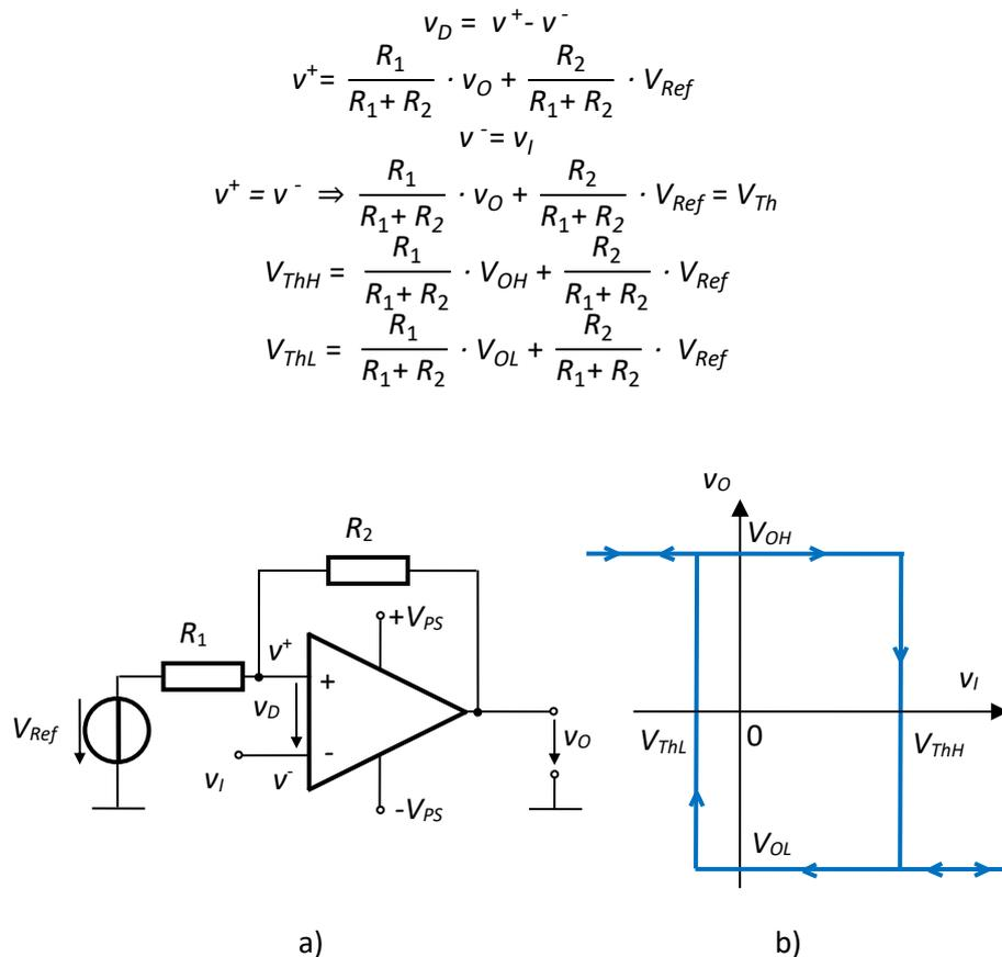
Fig.4.27. Inverting hysteresis comparator with asymmetric thresholds
