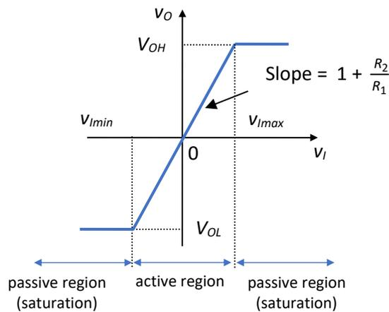
Fig.4.38. VTC  $v_O(v_I)$  for the noninverting amplifier
