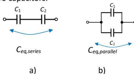
Fig.1.24. Capacitor connections a) series; b) parallel.
