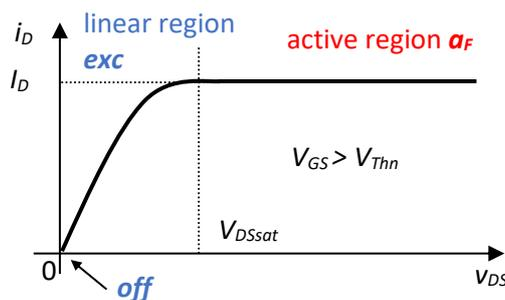
Fig.5.21. NMOS output characteristic  $i_D(v_{DS})$
