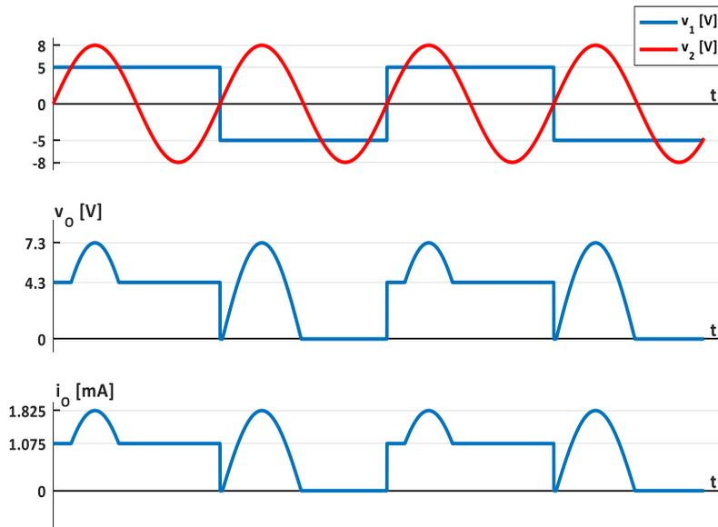
Fig.2.31. Waveforms for  $v_1(t)$ ,  $v_2(t)$ ,  $v_o(t)$  and  $i_o(t)$
