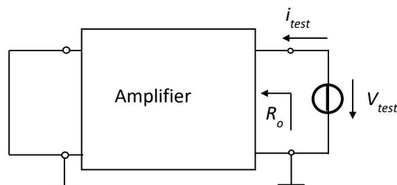
Fig.3.5. Circuit for computing  $R_o$
