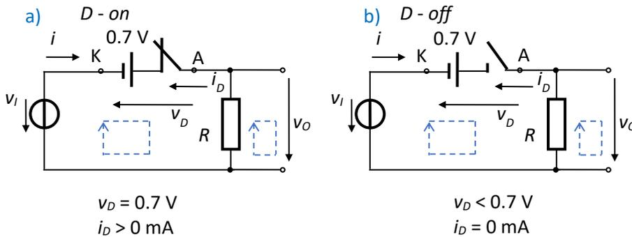
Fig.2.21. Equivalent schematics for a) *D - on*, b) *D - off*.
