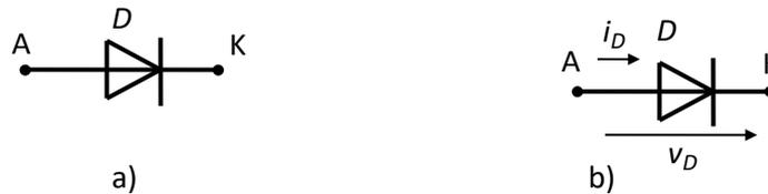
Fig.2.4. Semiconductor diode
