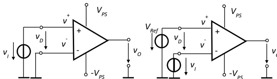
Fig.4.6. Simple comparators with op-amp: a)  $v_i = v^+$ ; b)  $v_i = v^-$ .
