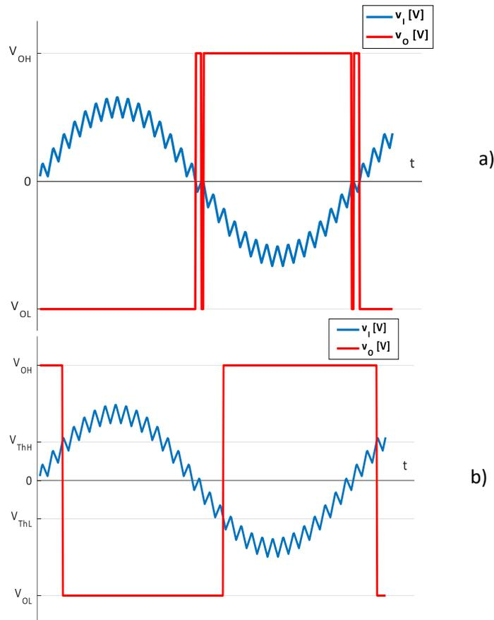
**Fig.4.22.** Waveforms for  $v_i(t)$  and  $v_o(t)$  for a noisy input
