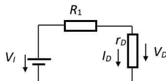
Fig.2.13. The dc equivalent circuit
