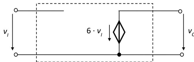
Fig.4.51. Model of the noninverting amplifier
