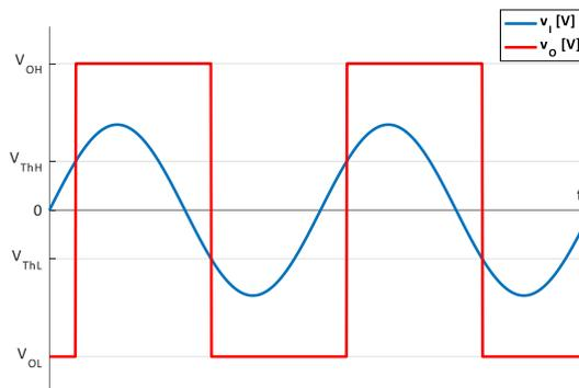
**Fig.4.26.** Waveforms for  $v_I(t)$  and  $v_O(t)$  for the noninverting hysteresis comparator with symmetric thresholds
