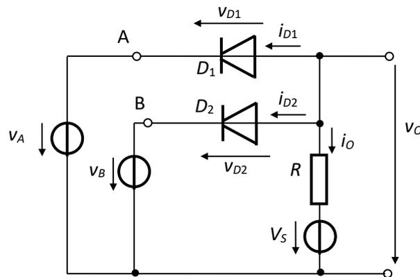
Fig.2.33. Spatial minimum multi-port circuit with  $V_{Omax} = V_S$
