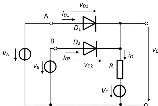
Fig.2.30. Spatial maximum multi-port circuit with  $V_{Omin} = V_C$
