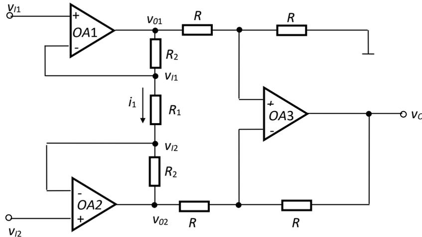
Fig.4.61. Instrumentation amplifier
