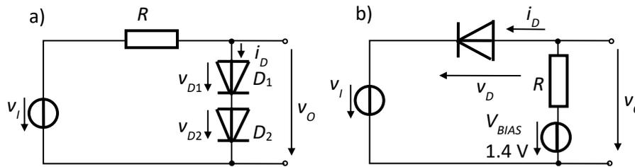
Fig.2.39. Superior voltage limiter,  $V_{Omax} = 1.4 \text{ V}$
