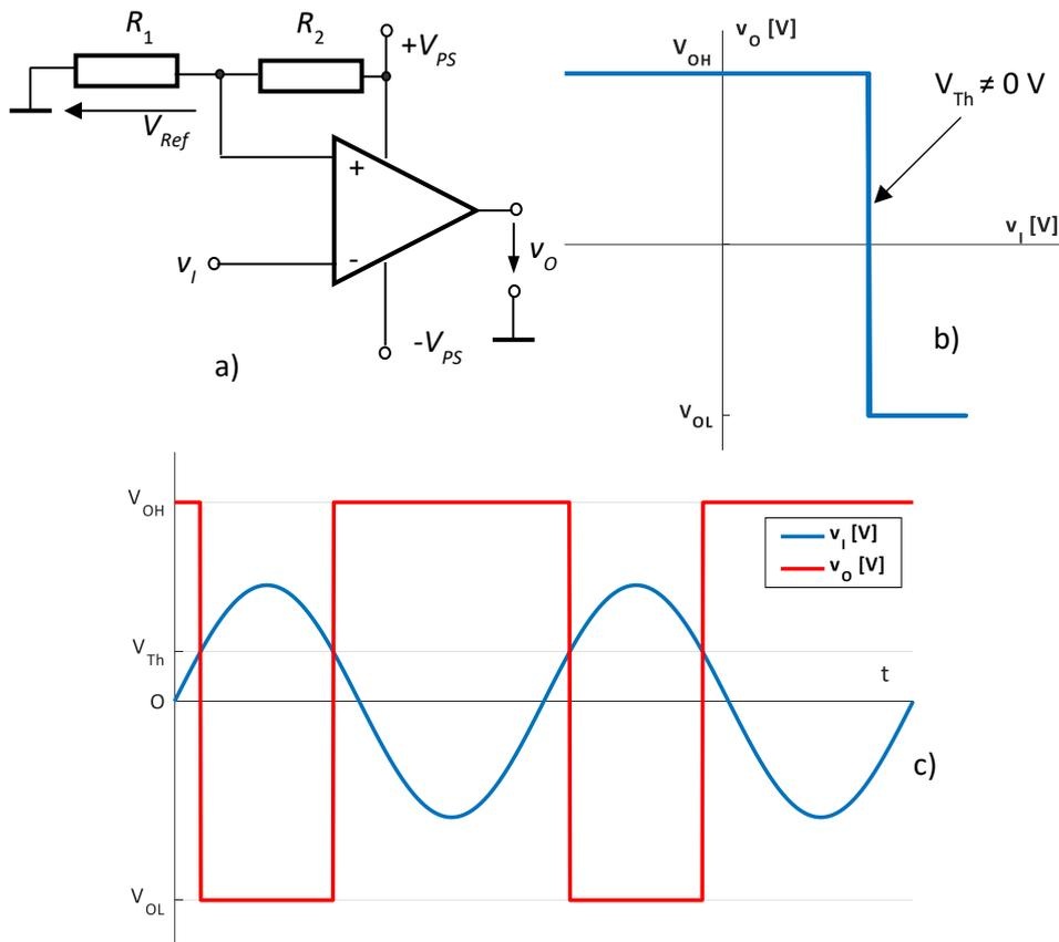
**Fig.4.13.** Simple comparator, inverting,  $V_{Th} \neq 0$  V
