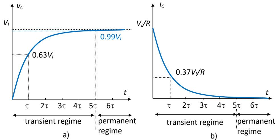
**Fig.1.26.** Waveforms for the circuit in Fig.1.25
