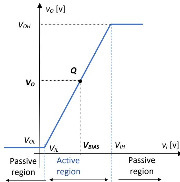
Fig.3.14. VTC  $v_o(v_i)$  for the voltage amplifier with unipolar supply
