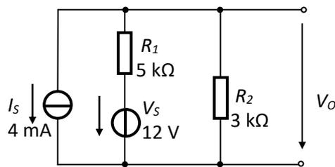
Fig.1.15. Superposition method - illustration
