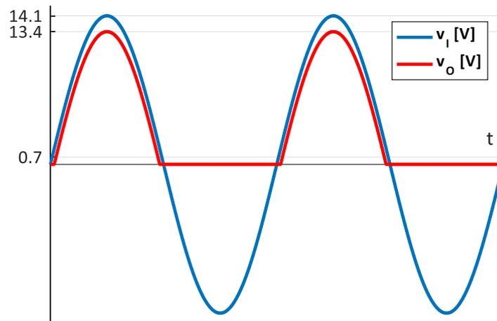
Fig.2.46. Half-wave rectifier - waveforms
