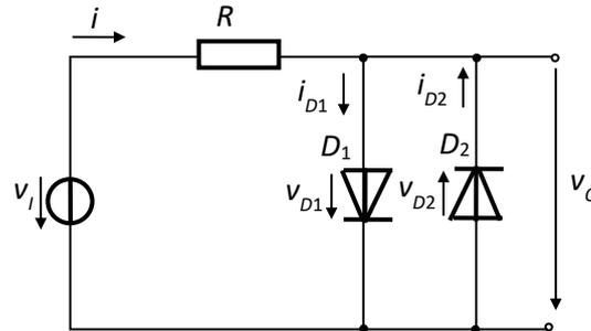
Fig.2.42. Double voltage limiter, to 0.7 V and -0.7 V
