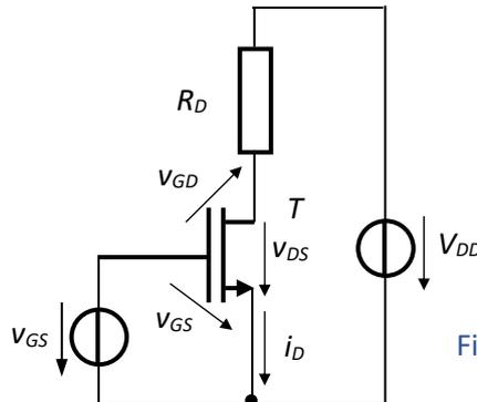
Fig.5.23. NMOS circuit
