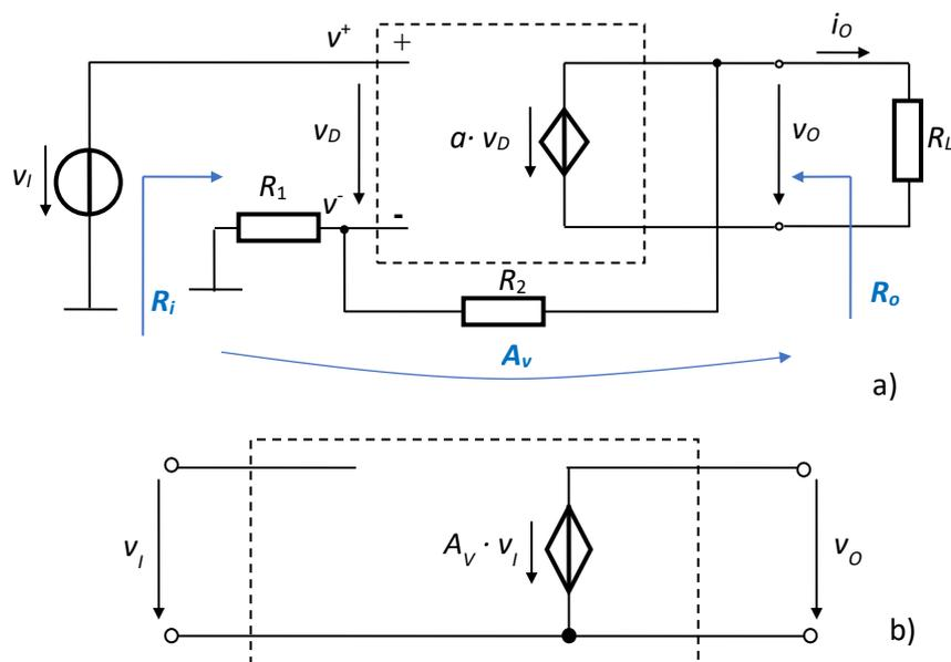
**Fig.4.39.** Modelling the noninverting amplifier as a VCVS
