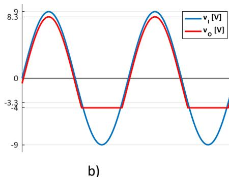
**Fig.2.41.** Inferior voltage limiter
