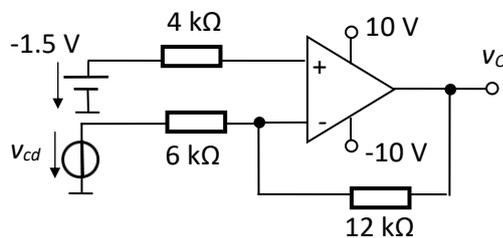
Fig.4.75. Inverting voltage domain converter – final circuit
