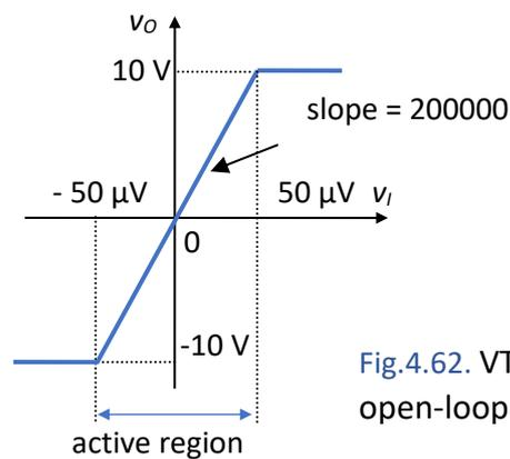
Fig.4.62. VTC  $v_O(v_D)$  of a finite open-loop gain amplifier
