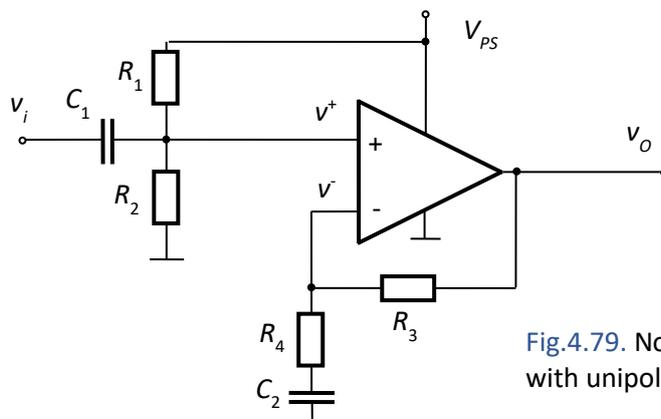
**Fig.4.79.** Noninverting amplifier with unipolar supply – final circuit
