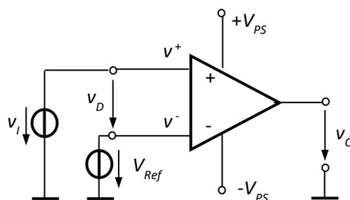
Fig.4.10. Simple comparator, noninverting, with  $V_{Th} \neq 0 \text{ V}$
