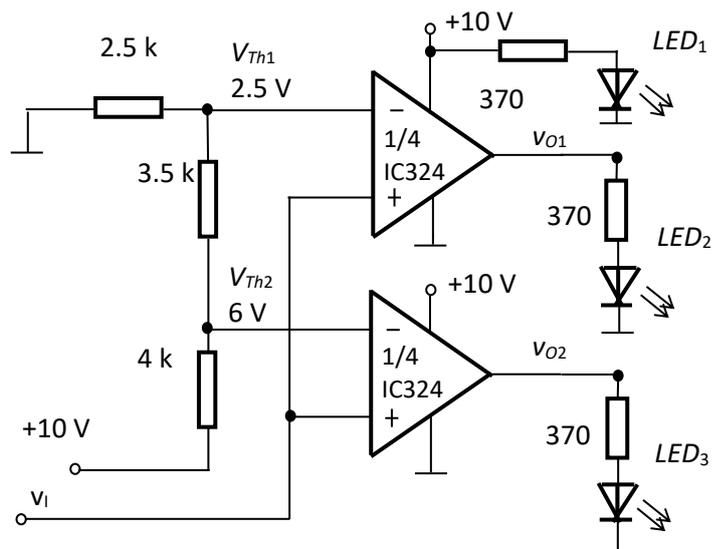
Fig.4.20. Optical voltage level indicator – LEDs gradually turn *on*
