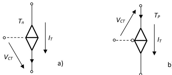
Fig.5.2. Voltage-controlled current source models for transistors
