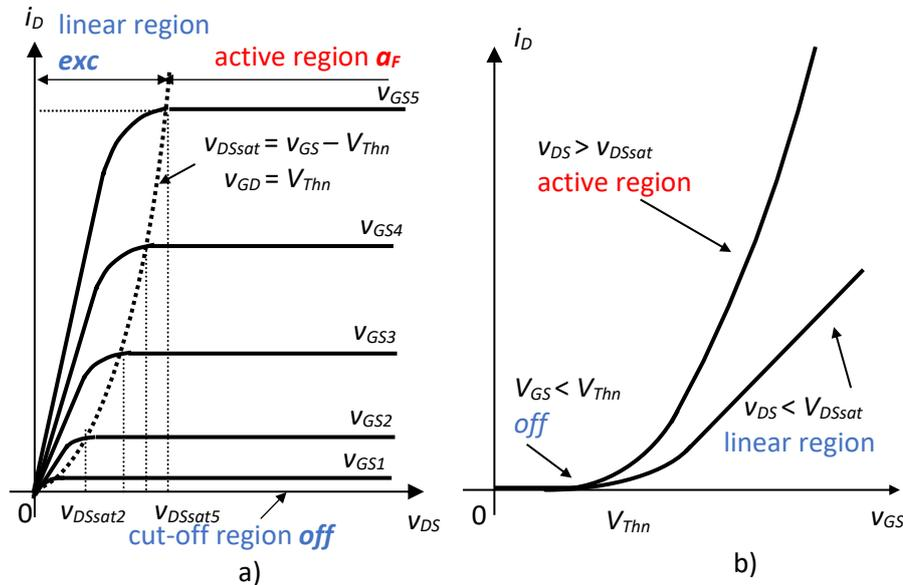
Fig.5.22. NMOS static characteristics
