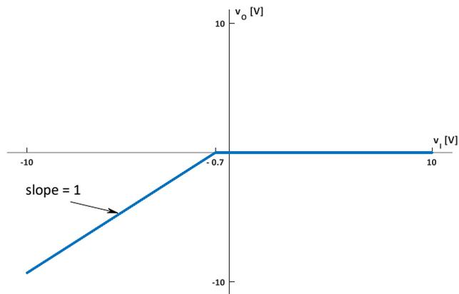
Fig.2.22. VTC  $v_o(v_i)$
