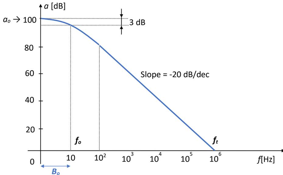
Fig.4.64. Gain-frequency plot of a general-purpose op-amp
