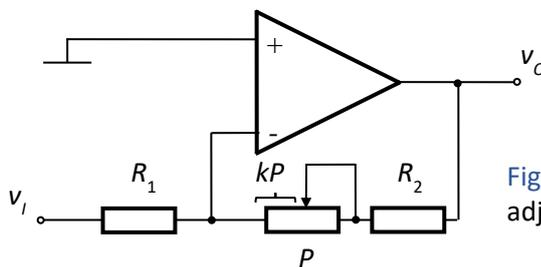
Fig.4.55. Inverting amplifier with adjustable gain – alternative solution
