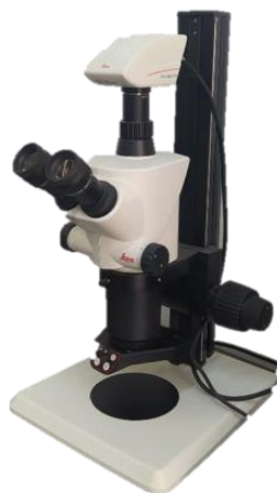
Fig. 5.20. Stereomicroscop optic tip Leica DNC2900
