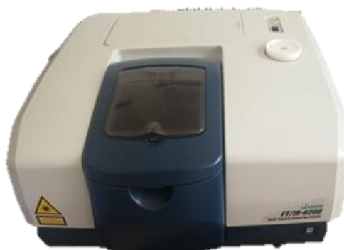
Fig. 5.18. Aparat Jasco FT/IR -6200 Fourier Infrared Spectrometer
