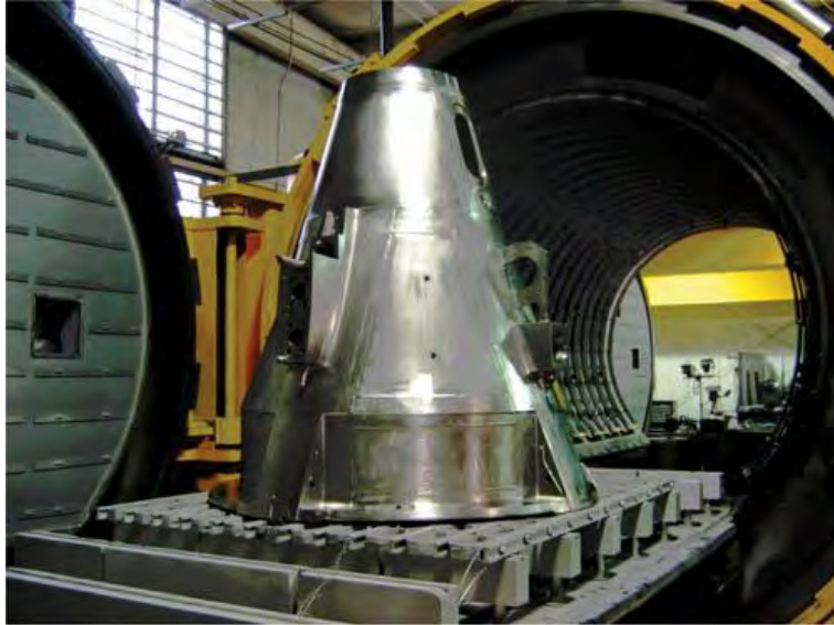
Vacuum stress relieving – to reduce residual stresses developed during fabrication. This titanium nosecone is stress relieved to minimize or eliminate forming and electron-beam welding stresses.
