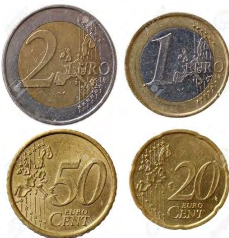
The 1 euro coin is composed of a silver-colored inner section (75% Cu, 25% Ni clad on nickel core) and a copper-colored outer section (75% Cu, 20% Zn, 5% Ni). The 2 euro has a reversed look and somewhat different composition: a copper-colored inner section (75% Cu, 20% Zn, 5% Ni clad on nickel core) and a silver-colored outer section (75% Cu, 25% Ni).
