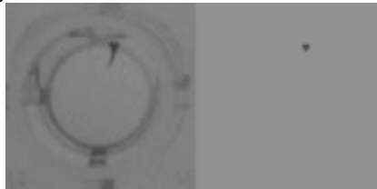
Figure 5.10 – Image segmentation made by PCNN classic model, on the right is the input and on the left the segmented image. It is able to discern the head of the fish from the rest of the image.
