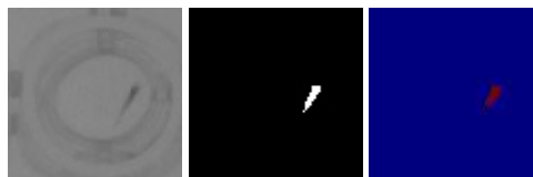
Figure 5.9 – Inference of a trained RandomForest Classifier for image segmentation. The left and middle image are the input image and mask used to derive new features and to train the model. The image from the right is the segmentation of the RandomForest Classifier.
