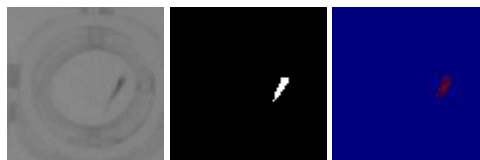
Figure 5.8 – Inference of a trained SVM model for image segmentation. The left and middle image are the input image and mask used to derive new features and to train the model and the right is the segmentation of SVM.
