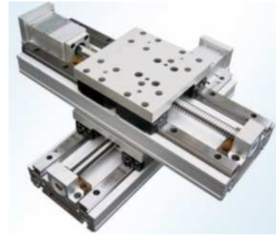
Fig. 2.16 Model de axe cinematice liniare X-Y pt. m-u CNC
