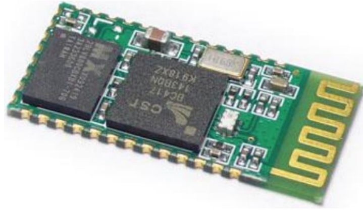
Fig. 5.9 – Modulul adaptor Bluetooth – Serial HC – 05 [5]
