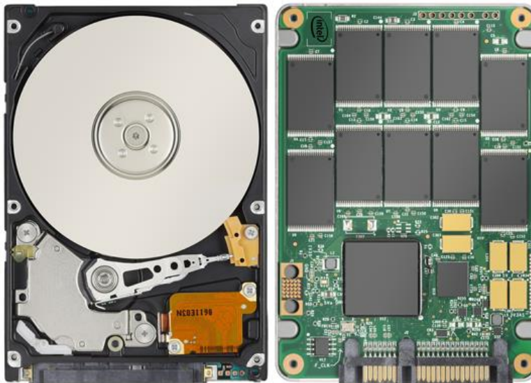
Figure 2.19. Classical hard disk (left) vs. solid state hard disk (right)
