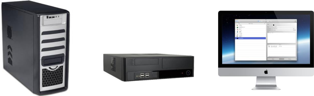
Figure 2.7. Tower case vs. desktop case vs. caseless PC
