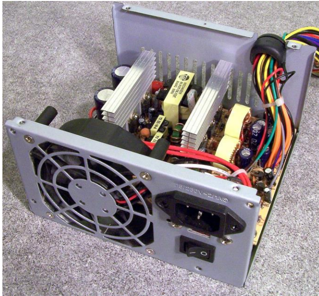
Figure 2.24. An ATX power supply unit with the cover removed
