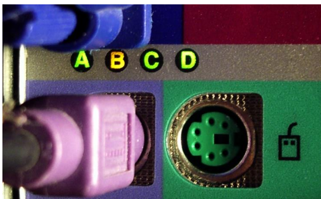
Figure 2.12. Diagnostic LEDs on the back pane of a PC
