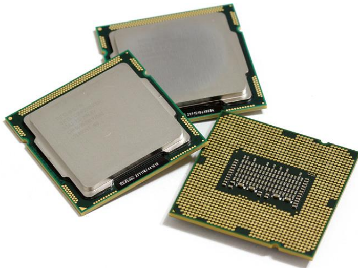
Figure 2.15. A CPU: Intel Core i5 750 (top and bottom view)
