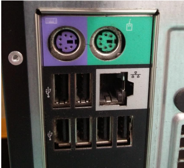
Figure 2.23. PS/2 connectors (violet - keyboards, green - mouse) and USB connectors below
