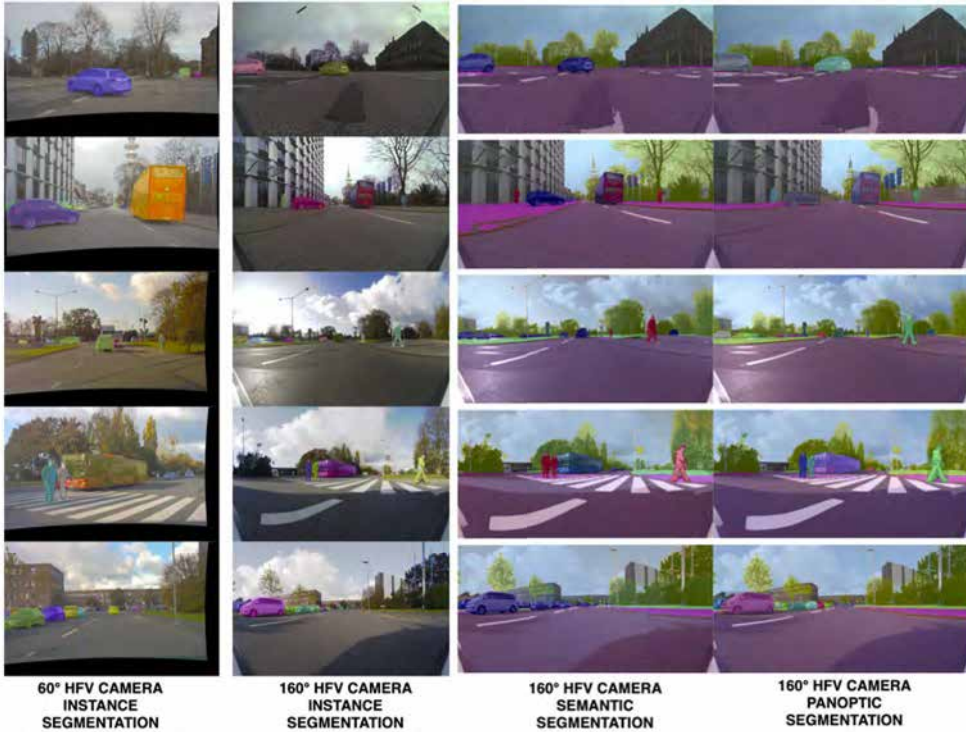
Figure 4.2: The front area of the vehicle is covered by two cameras: a narrow 60° horizontal field-of-view camera which provides instance segmentation at increased depth and a wider 160° horizontal field-of-view camera, which provides instance, semantic and panoptic segmentation for the near-range.
