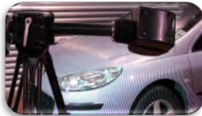
Fig.16.8. Sistemul Opti-Scan 350.10, InspecVision, [6].
