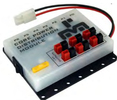
Fig. 6.80. Core Power Distribution Module
