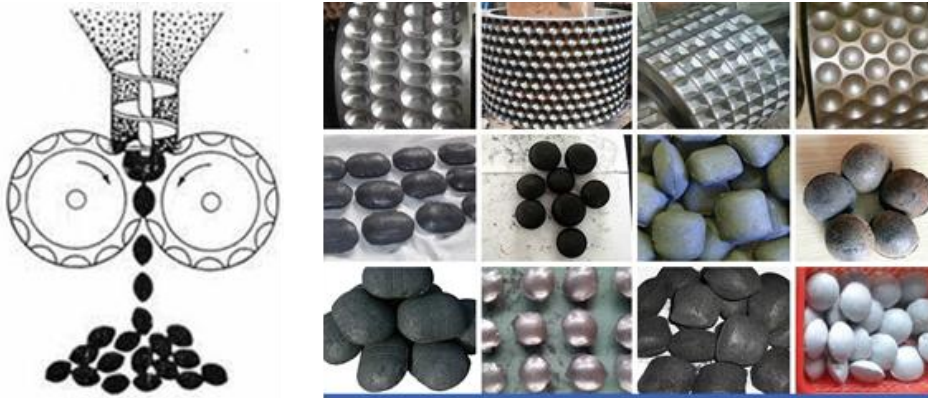
Figure 10. Briquetting process and different types (shapes and sizes) of briquets.
