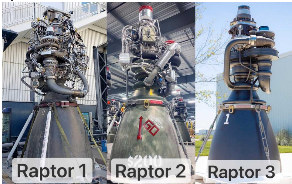
Figure 7. Design simplification of the Raptor rocket engine enabled by 3D printing [39]
