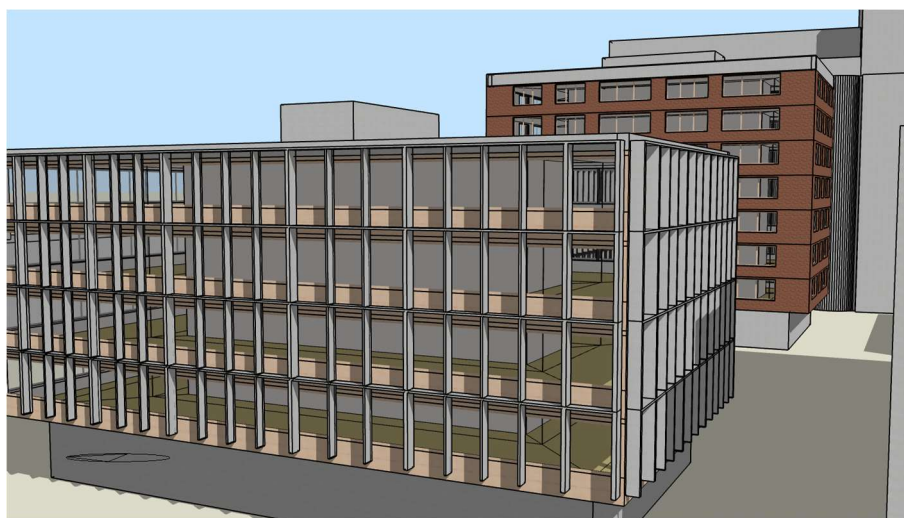
Figure 7.9 Detailed view of the used passive shading elements (horizontal and vertical overhangs) at the building B – geometry of the calculation model.
