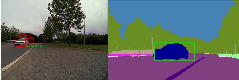
Figure 4.31. Example of successful validation. The super-sensor object is projected onto the RGB image in the left image. In the right image, the same object is projected onto the semantic segmentation image. The semantic classes' match is represented using green color.
