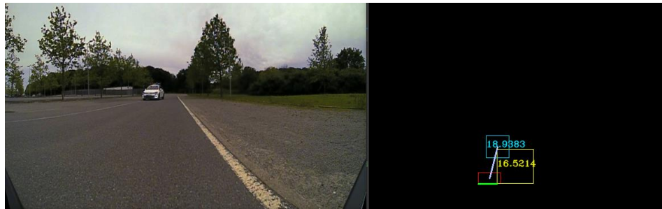
Figure 4.26. The correspondence between trifocal camera detections and measurements obtained from the LiDAR and RADAR sensors. The left-hand side of the figure presents the color image captured by the camera, while the right-hand side depicts the data association results for objects detected by the different sensing modalities.
