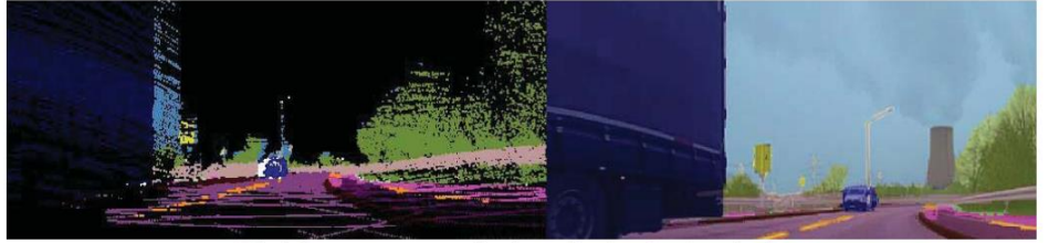
Figure 3.3. Issues that can appear when projecting LiDAR points onto the semantic segmentation image due to lack of synchronization.
