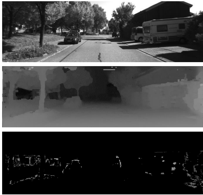
Figure 2.11. Disparity map (middle) of the proposed fusion and its error map(bottom) using a 2-pixel threshold of a KITTI image (top).
