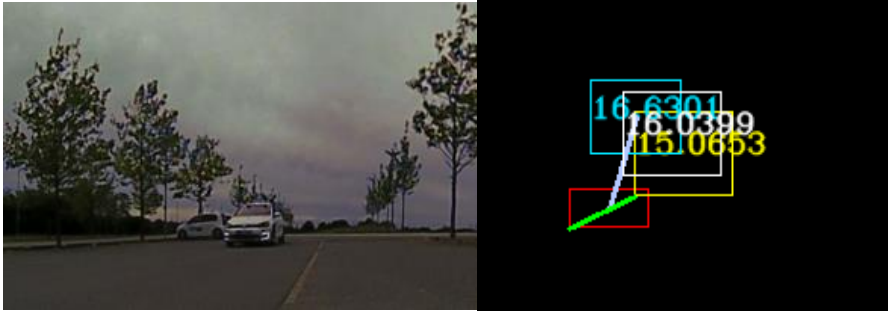
Figure 4.27. Associations between measurements originating from different sensors and their corresponding fusion results are illustrated in this figure. On the left-hand side, the RGB image is presented, while on the right-hand side, the data associations among the sensors are shown together with the resulting super-sensor object, which is depicted in white.
