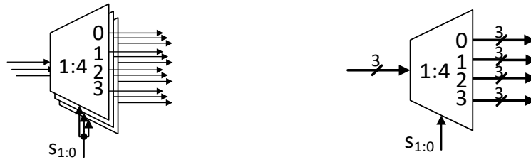
Figure 7. 2 The DMUX 1:4 unit with 3-bit datapath – implementation with three 1-bit DMUX 1:4 units (left) and the symbol (right)
