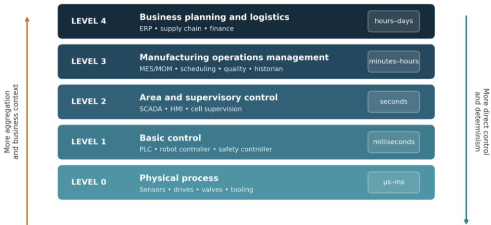
Figure 6.1. Five-level functional hierarchy: Level 0 represents the physical process and Level 4 business planning and logistics. The side arrows indicate increasing aggregation upwards and increasing control directness and determinism downwards.
