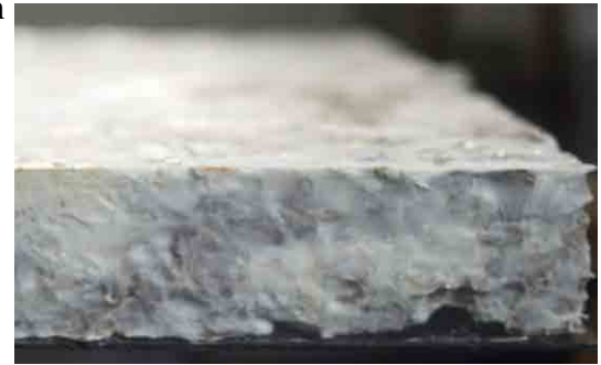
Fig 2 : Photo of the final result of the mycelium-based creation process [2]
